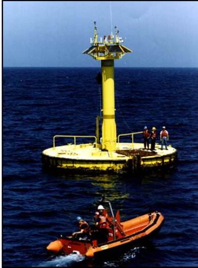
Figure 3-8. A 10-Meter Discus-Shaped Hull Buoy.
