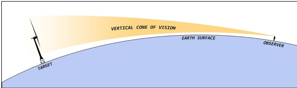
Figure 1. Effect of Earth Curvature on Visibility
