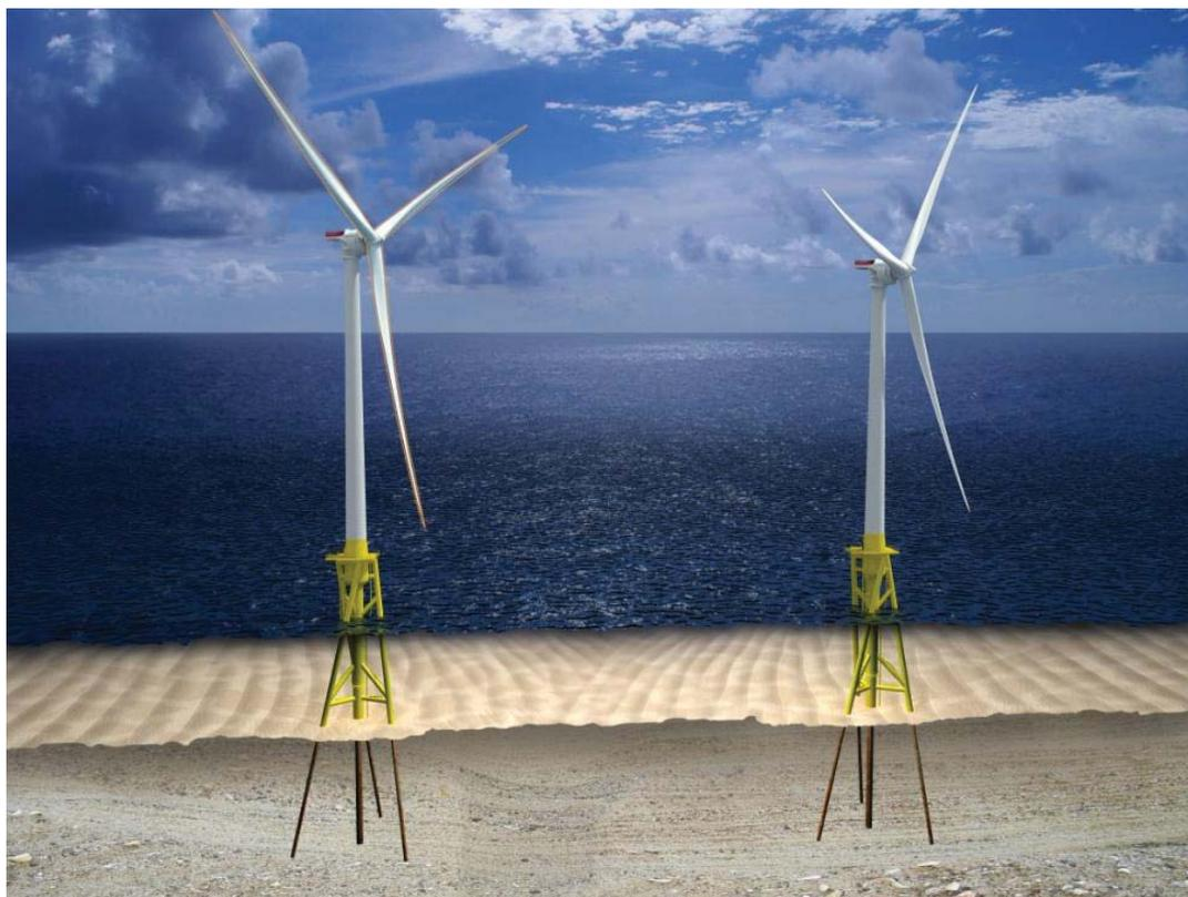
*Figure 2: Artist's rendition of VOWTAP turbines. Relative location depicted is conceptual; actual distance between turbines is likely to be between 6 and 12 rotor diameters, with tower centers between 600 and 1,200 meters apart. By comparison, an OCS sub-block is 1,200 m on a side.*
