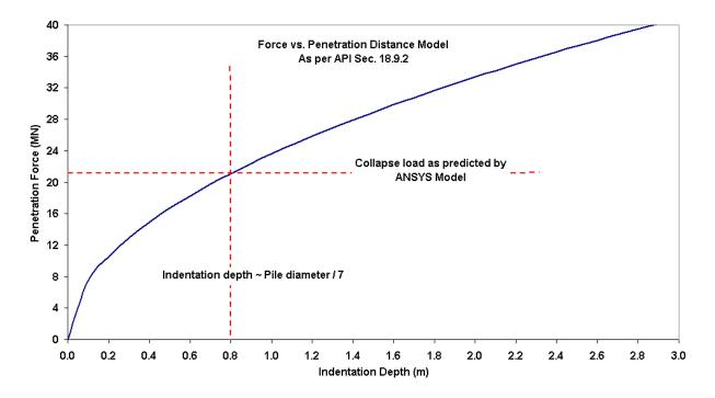
Figure 1: Load-indentation model utilized to model ship impact
