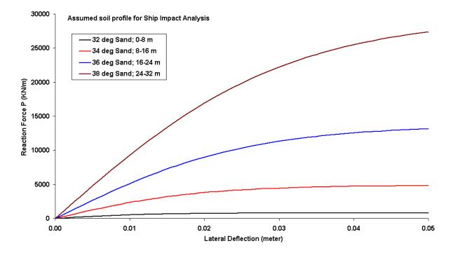
Figure 2: Assumed soil profile for the ANSYS model
