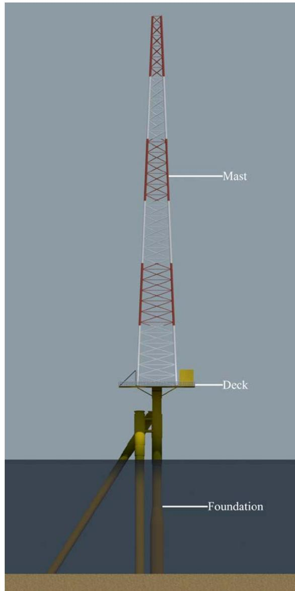
**Figure 2. Illustration of the meteorological tower braced caisson foundation, deck and mast (ESS Group, Inc. 2016).**
