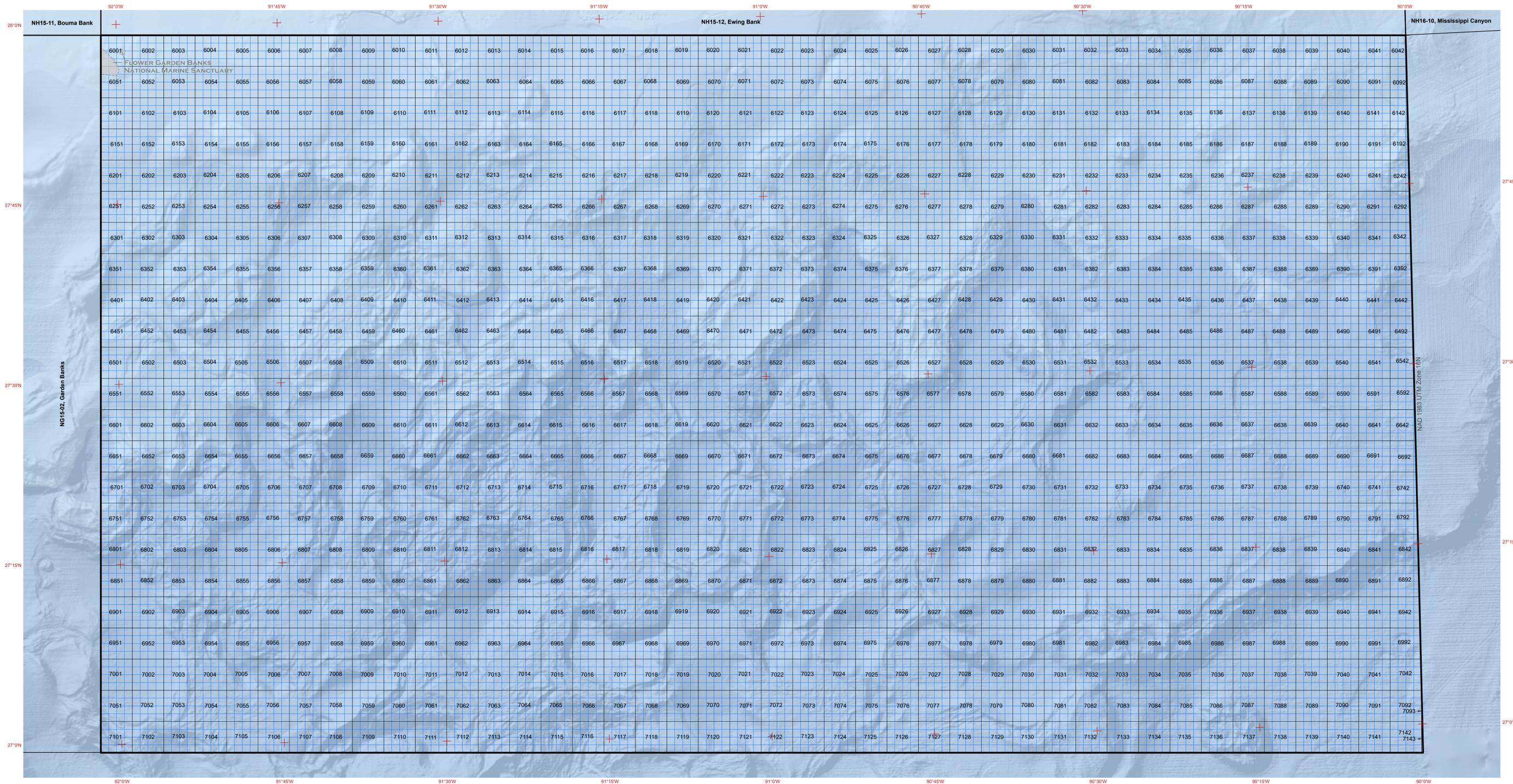
The boundaries of the regular aliquots are 1,200 meters on a side and contain 144 hectares. The regular boundaries are defined in terms of X and Y coordinates of the Universal Transverse Mercator Grid System based on the Geodetic Reference System (GRS), 1980 Ellipsoid.
