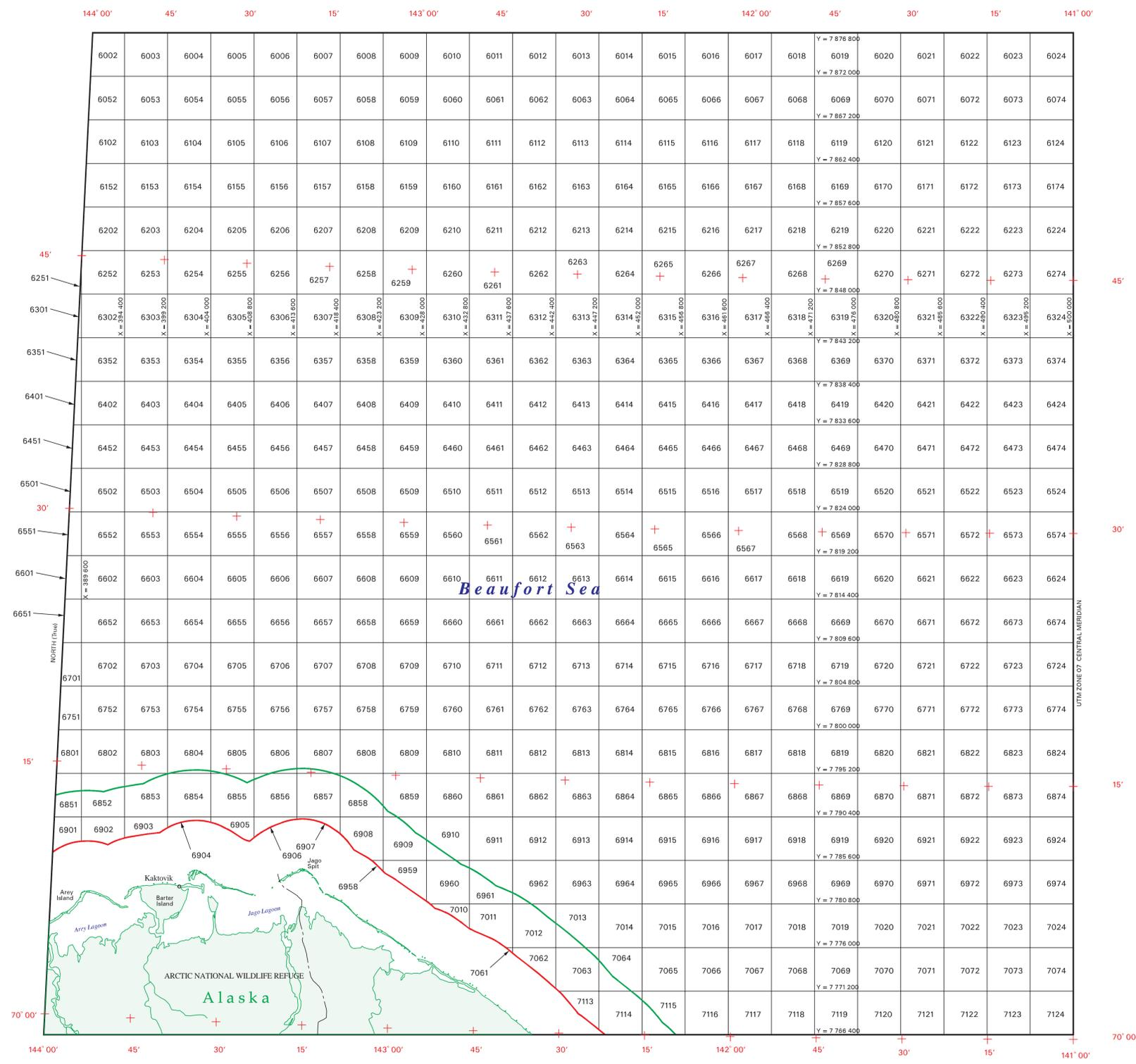
The boundaries of the regular blocks are 4,800 international meters on a side and contain 2,304 hectares. The regular boundaries are defined in terms of X and Y coordinates of the Universal Transverse Mercator Grid System based on the Geodetic Reference System (GRS) 1980 Ellipsoid.
