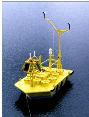
**Figure 3-5(b) 6-Meter Boat-Shaped Hull Buoy**
