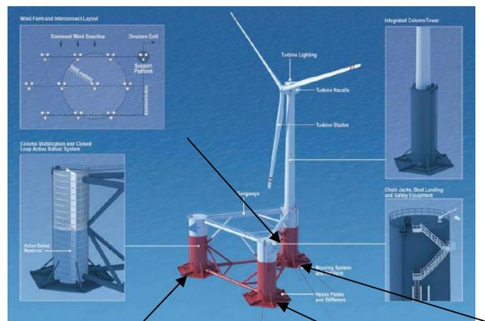
Figure 1: Principle Power Wind Float Technology. Arrows mark where anchor lines will come off of the floating platform.
