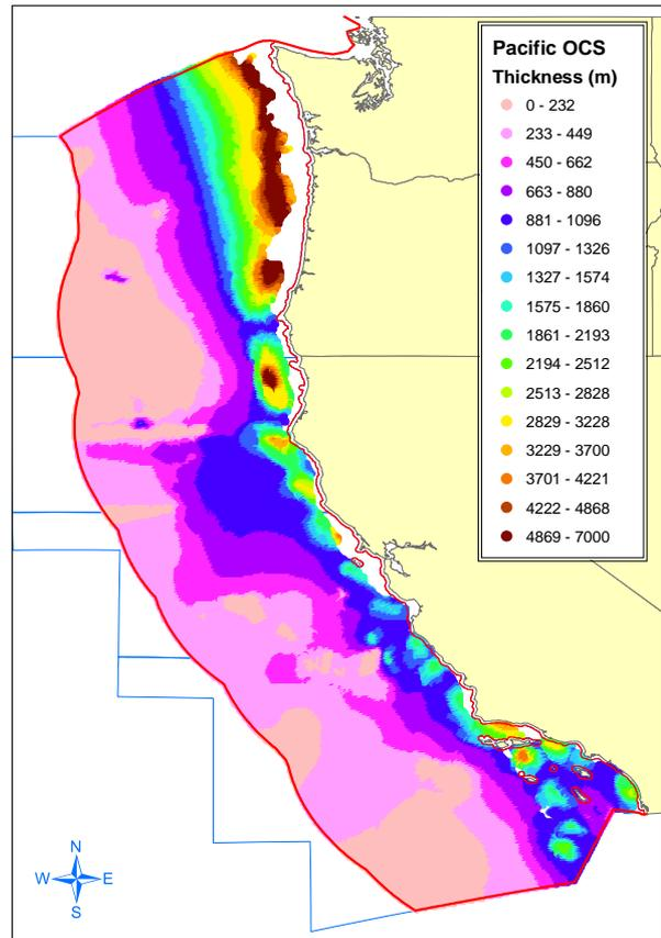
Figure 10. Sediment thickness input for the Pacific margin. Total thickness (shown here in meters) is divided equally into five stratigraphic units. (Figure modified after Collett, 1995 [3]).
