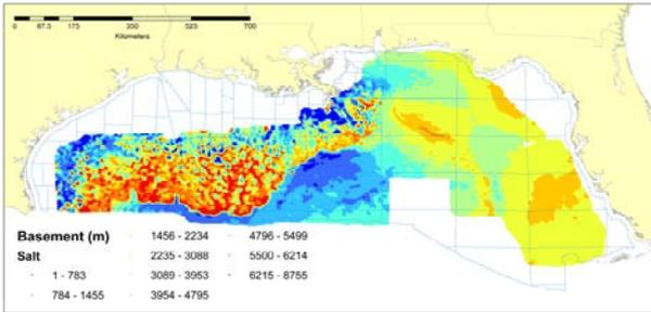
Figure 3. Depth to basement spatial input for the GOM. Thickness values are in meters.
