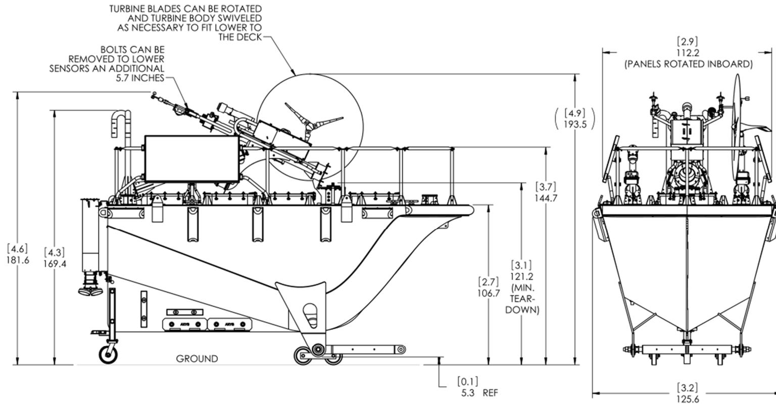
Figure 2: FLiDAR WindSentinel Dimensions – Transportation View
