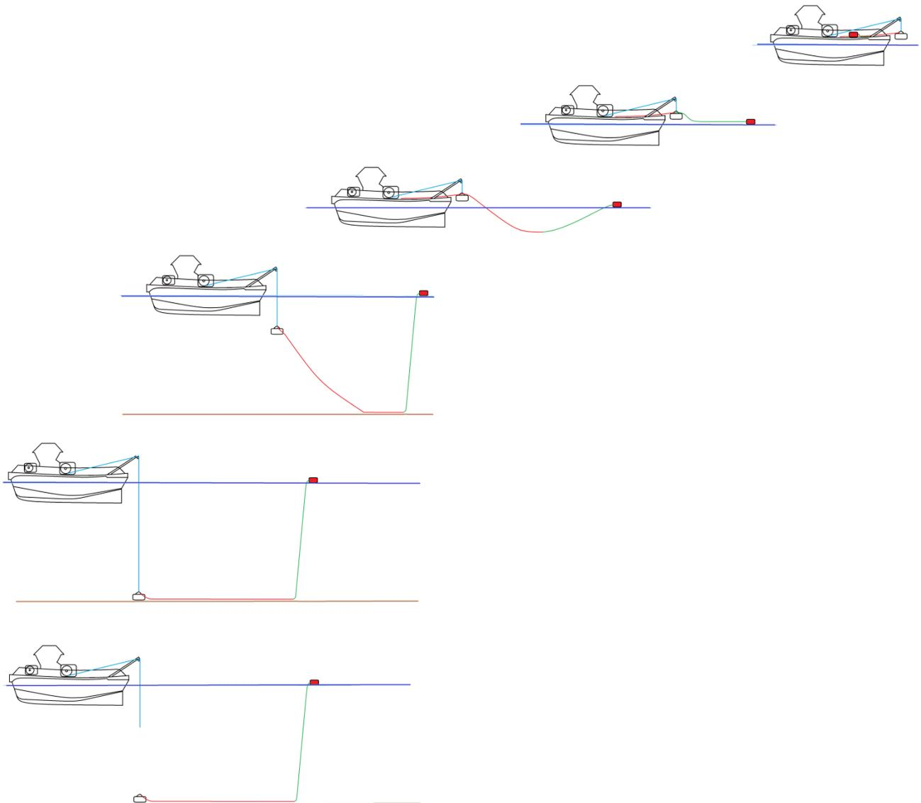
**Figure 3: Diagram of riser chain deployment operation. N.B. Image is not to scale; diagram to be used as a guide to operation only. Red lines refer to chain, green lines refer to ropes, light blue lines to winch wires.**
