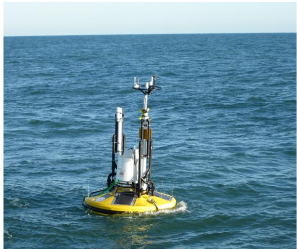
*Accurate measurement of wind profile using SEAWATCH Wind LiDAR Buoy*
