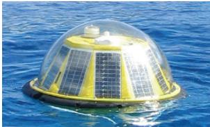
The AXYS TRIAXYS is a marine buoy measuring sea state conditions and sub surface currents.
