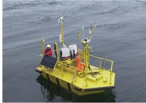
The AXYS WindSentinel is a marine buoy equipped with LiDARs specifically suited for marine conditions.
