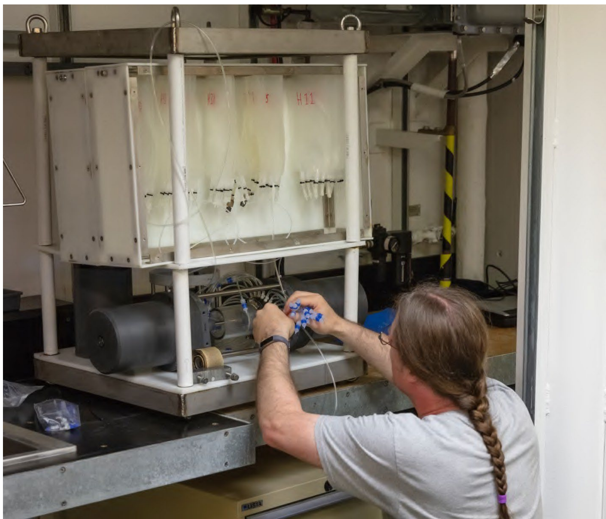
Setting up a moored Green Eyes water sampler. Roger Topp photograph.
