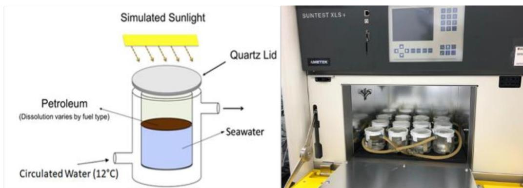
**Figure 4.** Experimental set-up of jacketed reaction beakers in Atlas Suntest XLS+.
