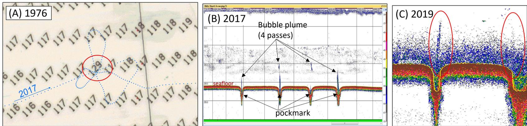
**Figure 24 (A) NOS smooth sheet #H09626 showing “anomalous” sounding (red circle). Blue line represents the shiptrack from a 2017 NMFS survey that passed over the anomaly 4 times. (B) Single beam read out during an NMFS bottom trawl survey in 2017 aboard the *F/V Ocean Explorer* showing imaged bubble plume along shiptrack in (A). (C) Closeup of sonar readout with water column anomalies still active in 2019 (red circles)**
