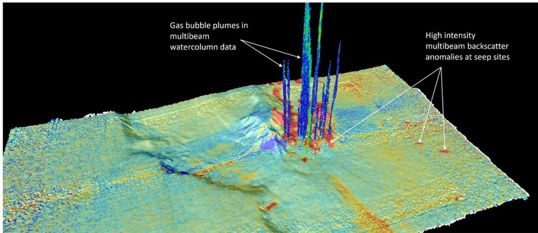
**Figure 51. Perspective view of multibeam bathymetry draped with water column and seafloor backscatter data. Warm colors represent high backscatter intensities, cool colors represent low backscatter intensities.**
