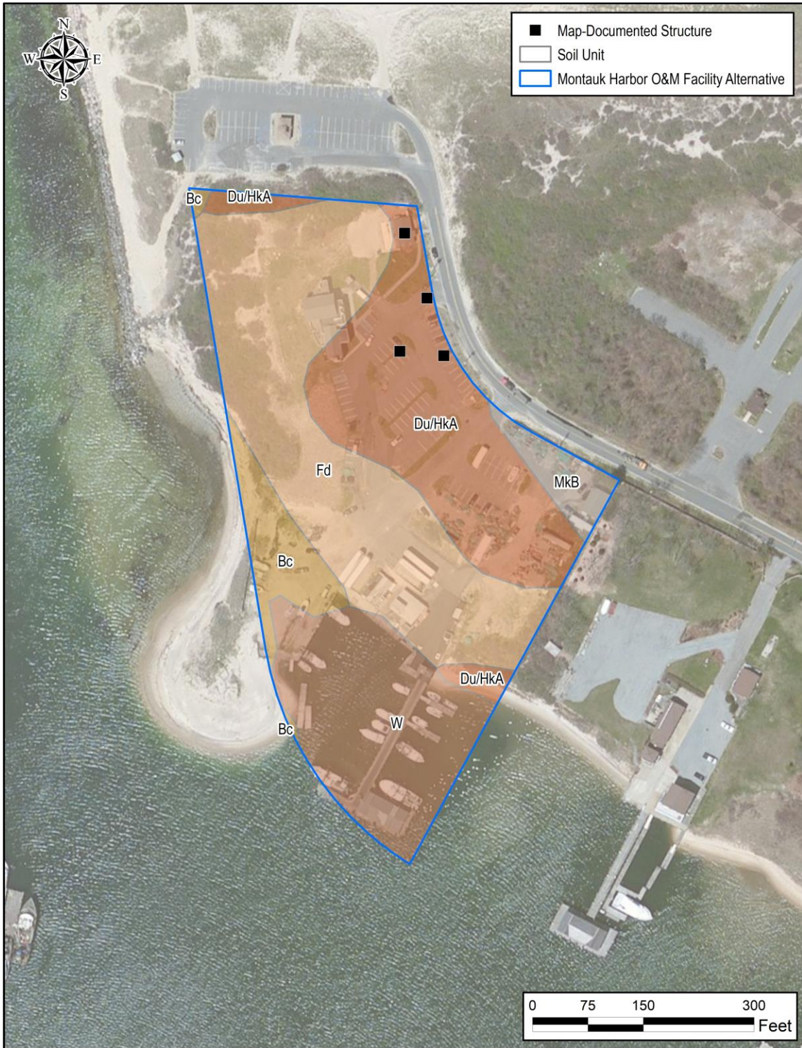
Inset 2.2-1. Map-Documented Structures and Soil Units within the Montauk Harbor O&M Facility Site.
