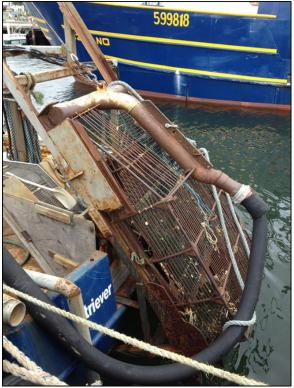
Figure 2.19: Hydraulic clam dredge before deployment
