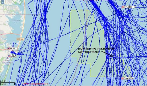
**Figure 5.1:** AIS traffic during a period of low fishing, 24-31 March 2021. Coastal transport routes are evident midway between shore and the western boundary of the Lease Area. Cargo vessel traffic is dominant in the eastern part of the Lease Area. The dense track from east to west in the SE part of the Area is a slow-drifting Greek tanker (Source: Sea Risk Solutions/Siitech WebVTS)
