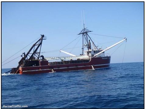
Figure 2.18 Hydraulic clam dredge fishing vessel in operation
