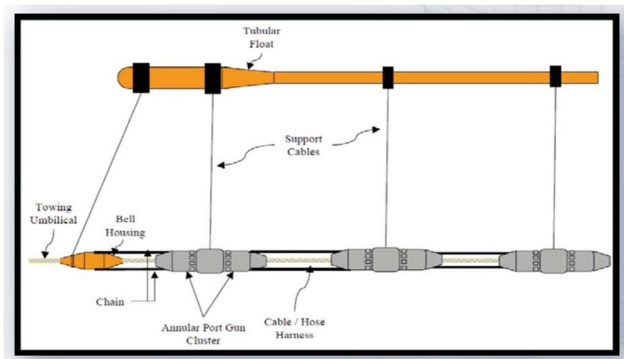
Figure 1-6. APG Sub-Array Sound Source (Example)
