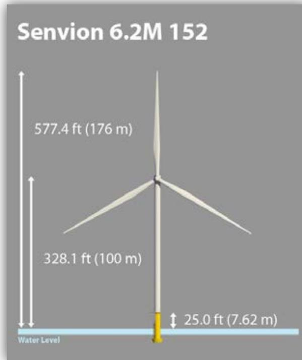
Figure 3–1. Wind turbine generator elevation schematic
