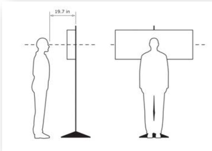
**Figure 6–2. Accurate viewing conditions for a TrueView™ simulation**
