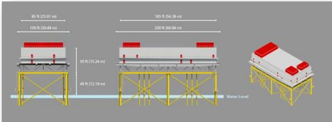
**Figure 5–2. Schematic of the substation and associated specification used in photosimulations**
