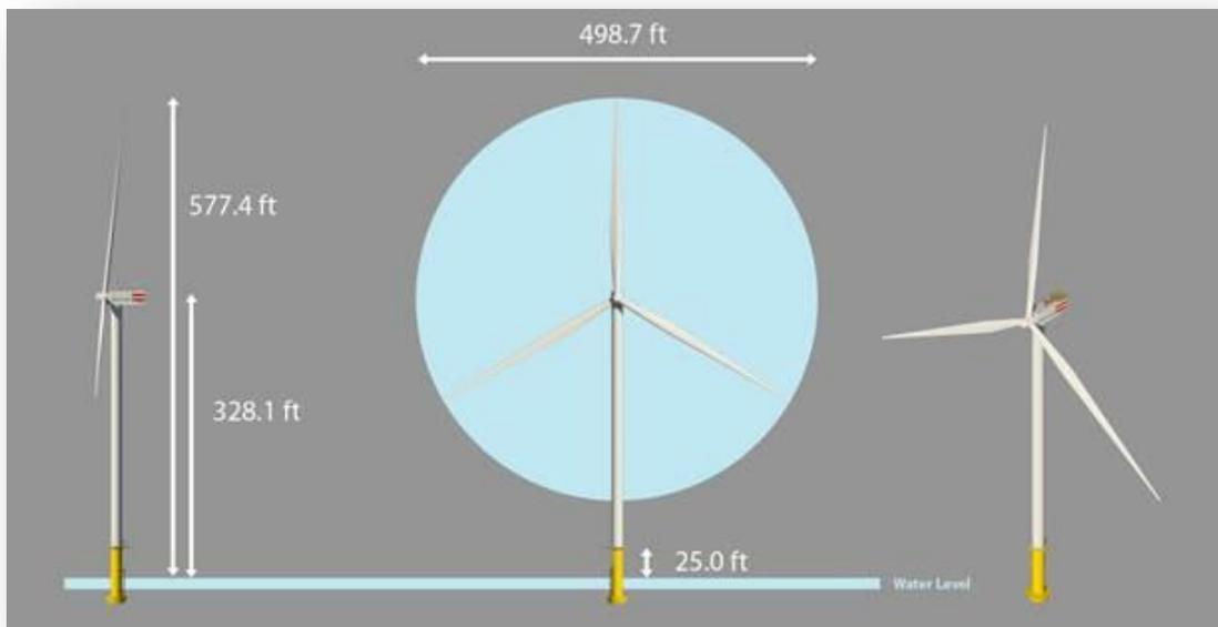
**Figure 5–1. Schematic of the Senvion 6.2M 152 Wind Turbine and associated specifications used in photosimulations**
