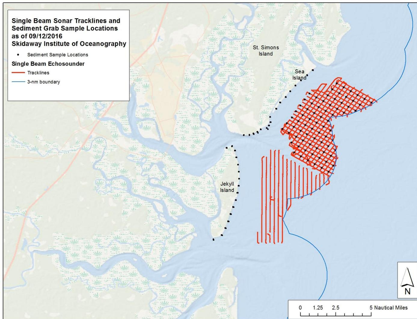
**Figure 5: Survey area of Georgia Sea Grant project in front of Jekyll, St. Simon's and Sea Islands. Bottom sediment grabs and beach samples are being collected, and single beam echosounding is being conducted, in summer 2016 and will be conducted in summer 2017 to highlight sediment transport pathways and locate beach compatible sand.**
