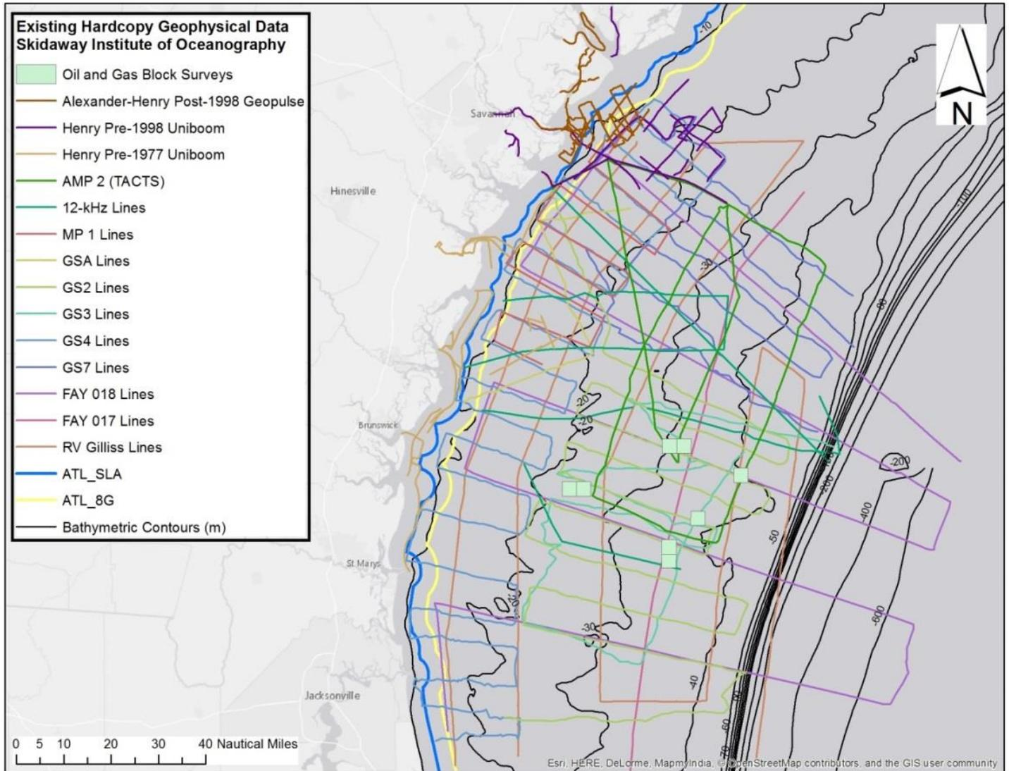
**Figure 3: Track lines of legacy geophysical datasets existing in the archives at the Georgia southern University Applied Coastal Research Laboratory on Skidaway Island. Note that few lines cover the 3-8 nm region of interest.**
