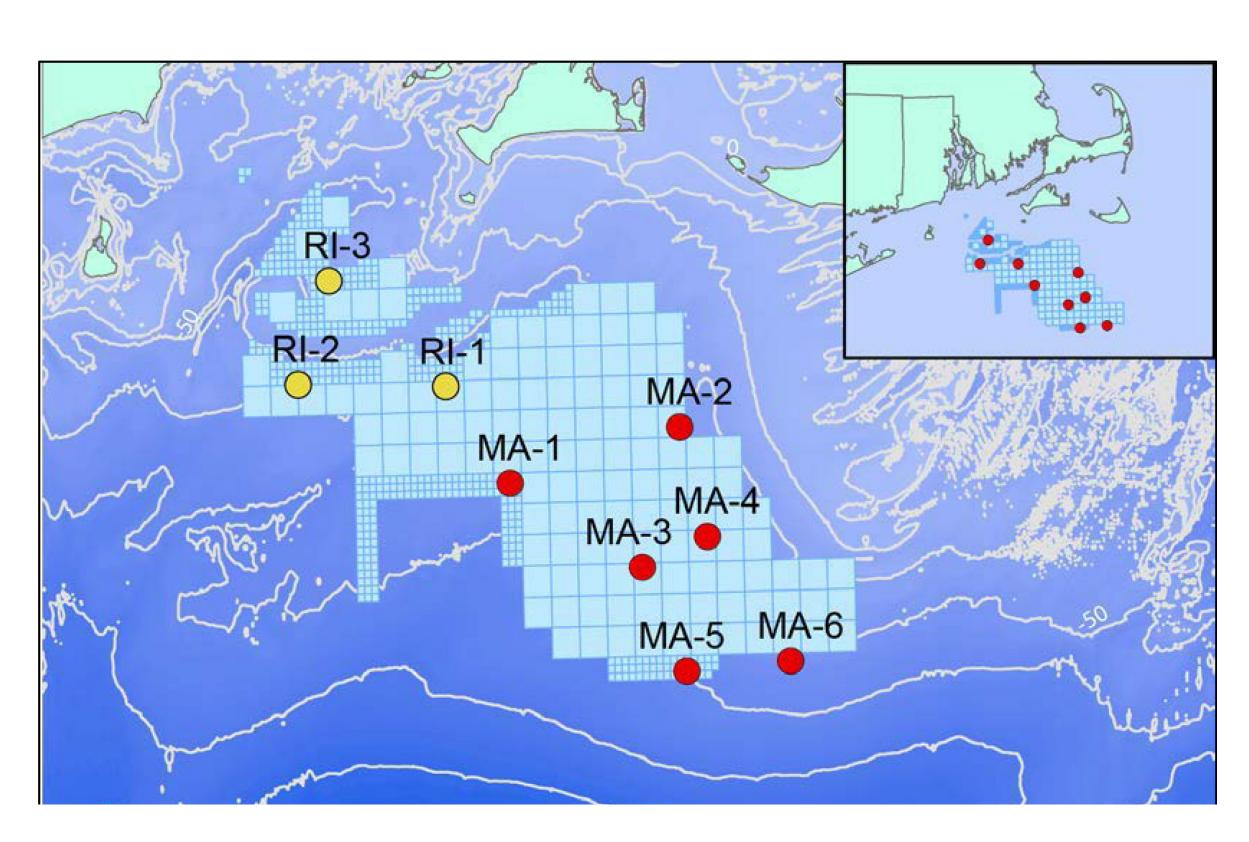
Recording sites (red and yellow dots) in the MA and RI wind energy areas, from November 2011 to March 2015. Ambient sound levels across all sites varied between 96 dB and 103 dB re 1 µPa in the hearing range of baleen whales during 50% of the recording time. These measurements were part of a cooperatively funded study by BOEM and MassCEC. (www.boem.gov/RI-MA-Whales-Turtles)
