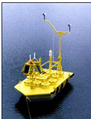
Figure 3-8b 6-meter Boat-shaped Hull Buoy
