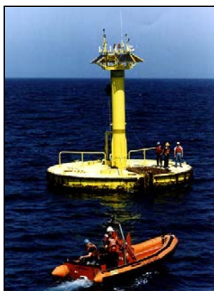
Figure 3-8a 10-meter Discus-shaped Hull Buoy
