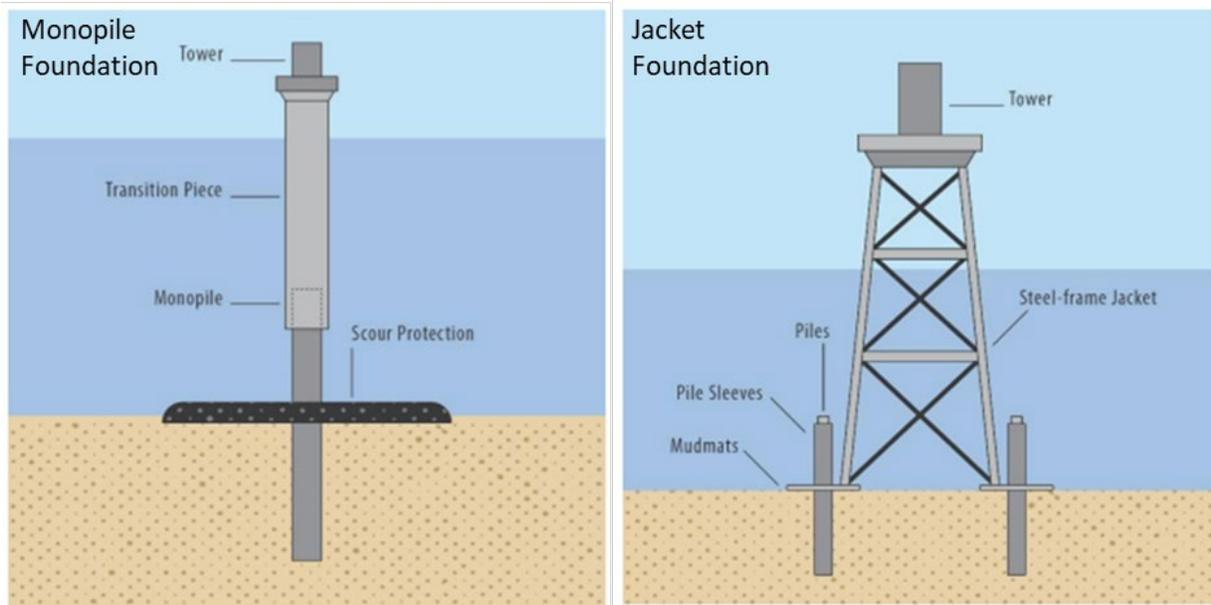
**Figure 7. Examples of Monopile and Jacket Foundations**
