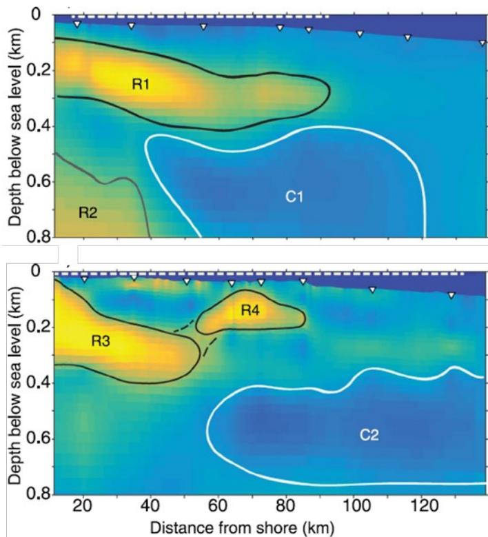
Imagery taken from the shoreline to the edge of the OCS using a controlled source electromagnetic system combined with a magnetotelluric method to identify salinity levels in groundwater offshore.
