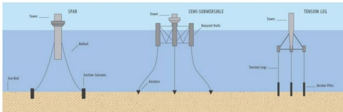
**Figure 8. Examples of Floating Turbine Anchor Foundations**
