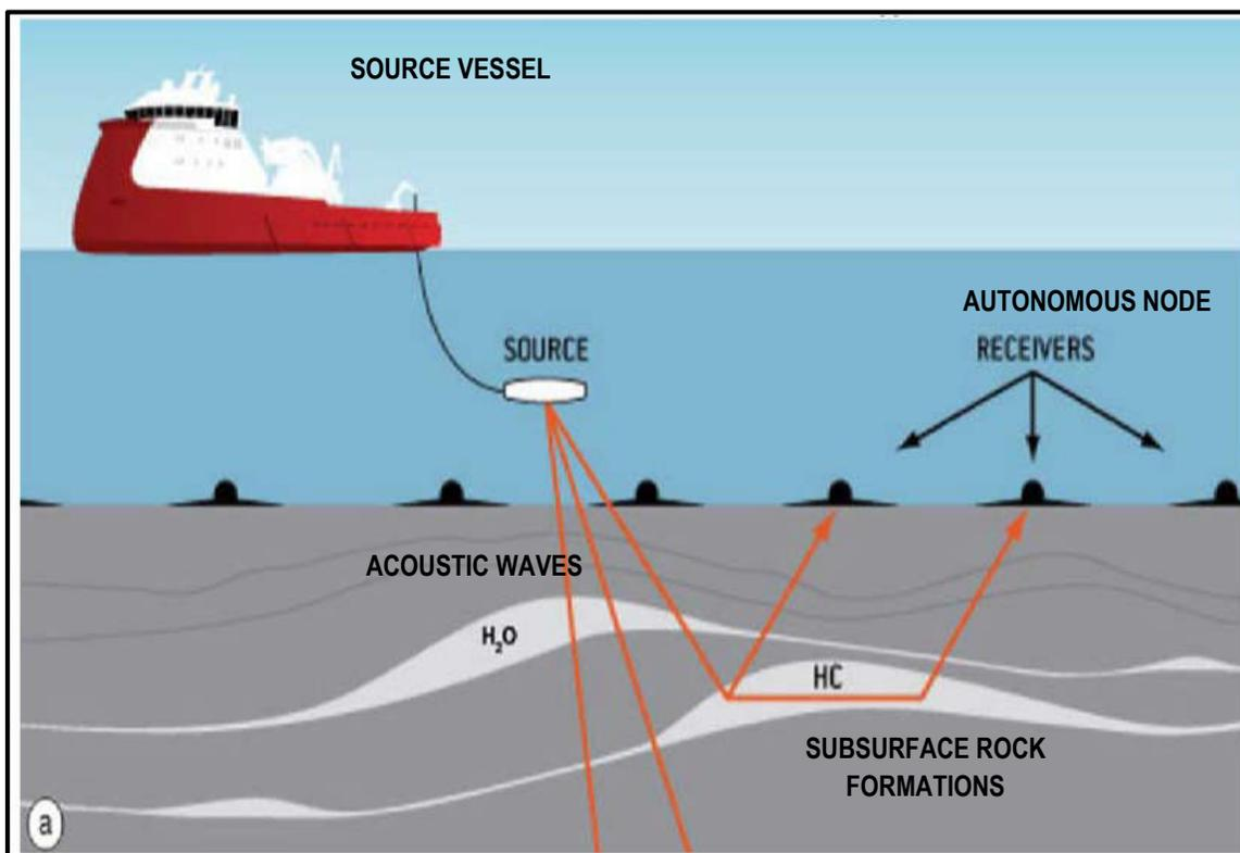
**Figure 1-3. Illustration of the Nodal Marine Geophysical Subsurface Survey**
