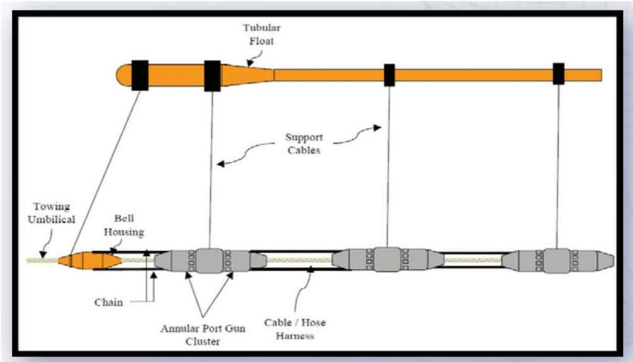
Figure 1-6. APG Sub-Array Sound Source (Example)
