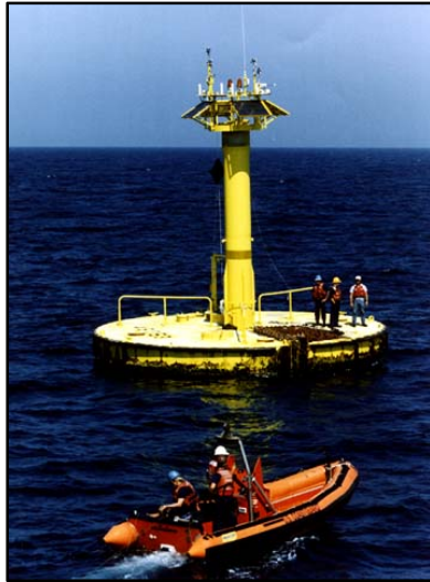
Figure 3-8. A 10-Meter Discus-Shaped Hull Buoy.
