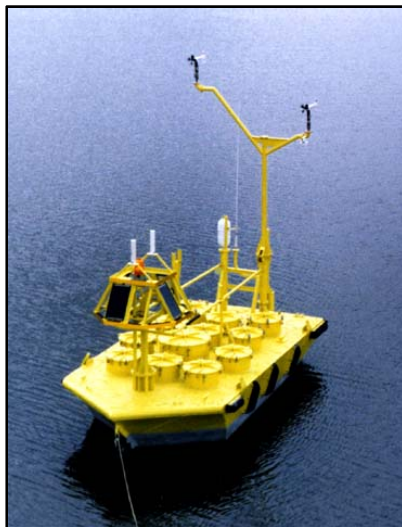
Figure 3-9. A 6-Meter Boat-Shaped Hull Buoy (also known as a NOMAD).
