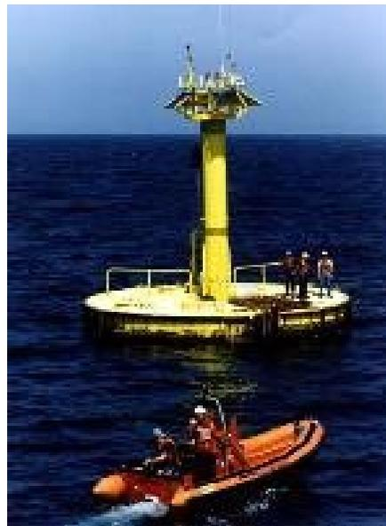
**Figure 2-4: 10-Meter Discus-Shaped Hull Buoy**
