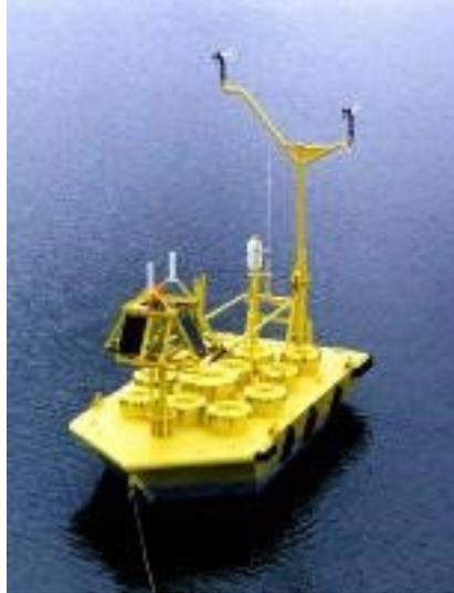
**Figure 2-5: 6-Meter Boat-Shaped Hull Buoy**
