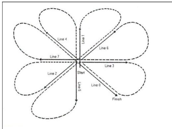
Figure 18 - USBL Calibration Pattern
