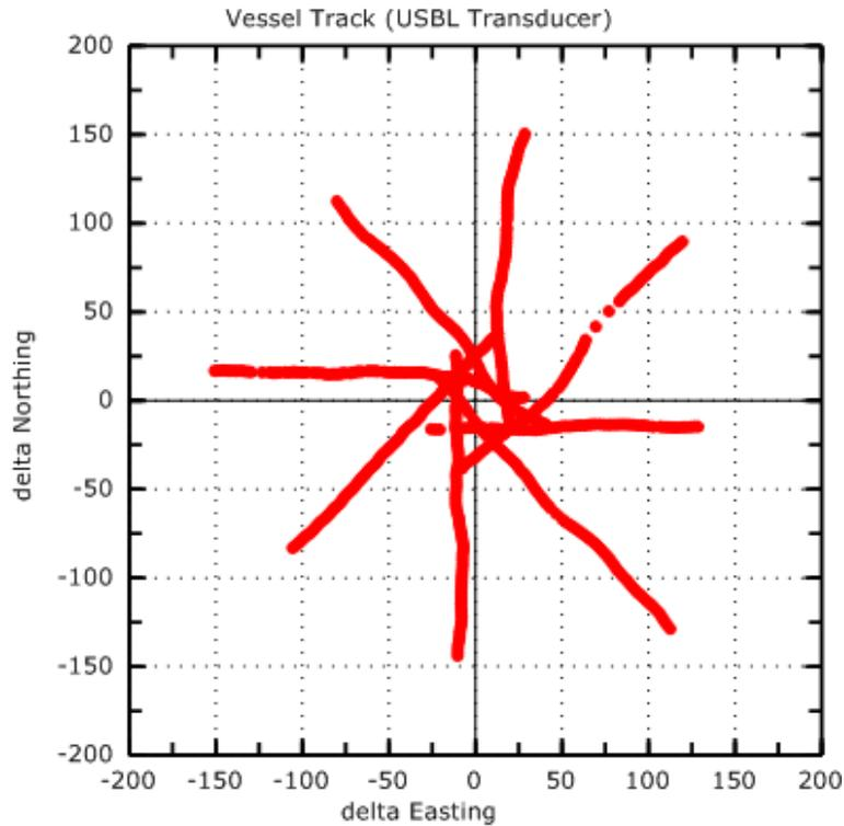
Figure 19 - USBL Calibration Lines
