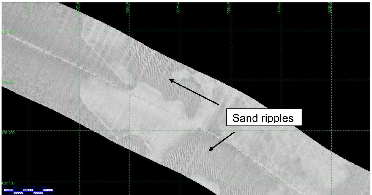
Figure 16 - Side Scan Sonar Check
