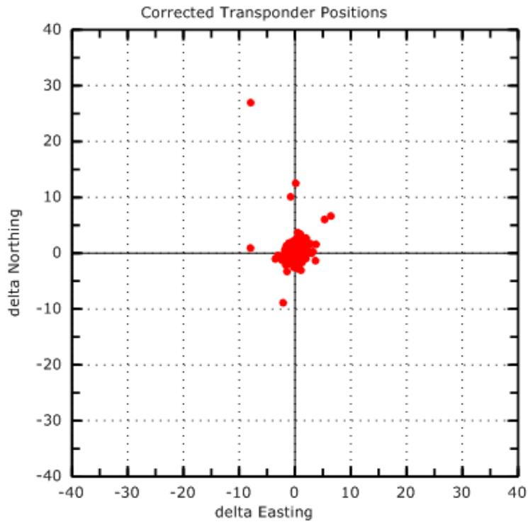
Figure 21 - USBL Calibration Positions Post-Cal
