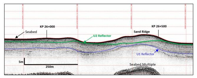
Figure 9.15 Sub-bottom Profile showing Sand Ridge
