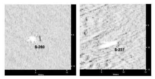
The seabed between KP 18+000 – 22+000 is predominantly fine to coarse sand with some gravel (Medium Reflectivity). From KP 22+000 – 24+500 the bottom is characterized by mixed sediments (silt-clay to sand and gravel; Variable Reflectivity), with several areas of Medium-High Reflectivity (coarse sand, gravel, cobbles and possible boulders). The Variable Reflectivity areas again correlate to the irregular seabed areas as seen in the bathymetry data.
