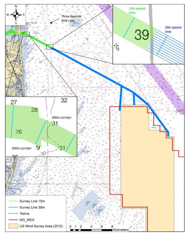
Figure 6.1 Offshore export cable survey line plan
