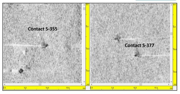
Figure 10.3 Side scan Imagery of two sonar contacts with greater than 1 m relief between KP 0+000 and KP 9+000
