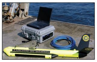
Aboard the RV *Shearwater* the towfish height off seafloor was maintained at 10-20% of the sweep range using a deck mounted hydraulic winch and armored cable. The towfish position was calculated in realtime using the USBL system. A backup positioning system was also used, utilizing a digital cable counter sheave to measure cable out from the stern of the vessel.
