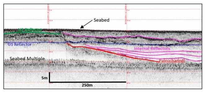
Figure 9.10 Northwest Flank of Paleochannel near KP 9+000
