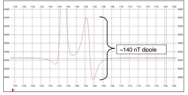
Figure 6.8 Geometrics G-882 Magnetometer Data Example
