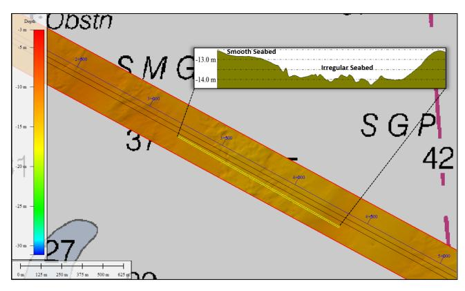
Figure 9.4 Bathymetry between KP 3+000 – 4+500 Showing Transition From Smooth to Irregular Bottom
