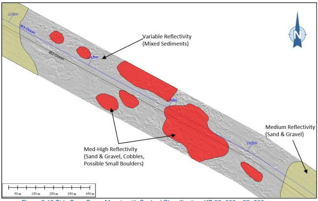
Figure 9.12 Side Scan Sonar Mosaic with Seabed Classification, KP 22+000 – 23+900
