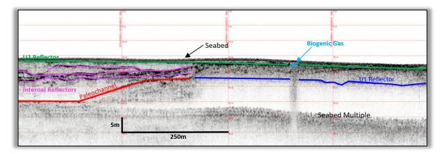
Figure 9.3 Sub-bottom Profile with Mapped Reflectors
