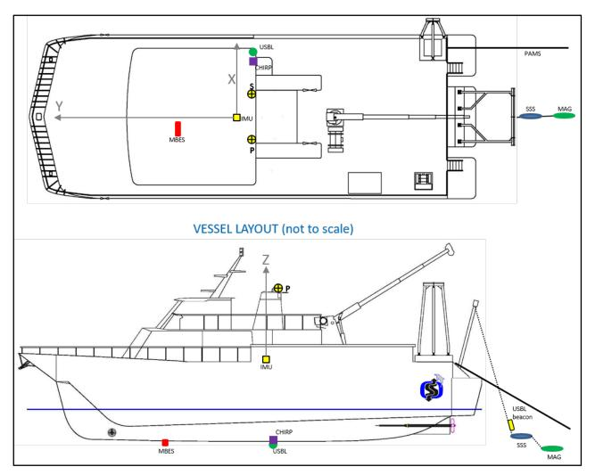
Figure 6.3 RV Shearwater HRG Offset Diagram
