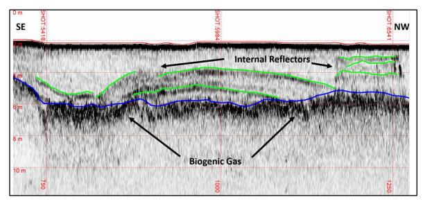
Figure 10.1 Sub-bottom profile showing reflector types on inshore cable route
