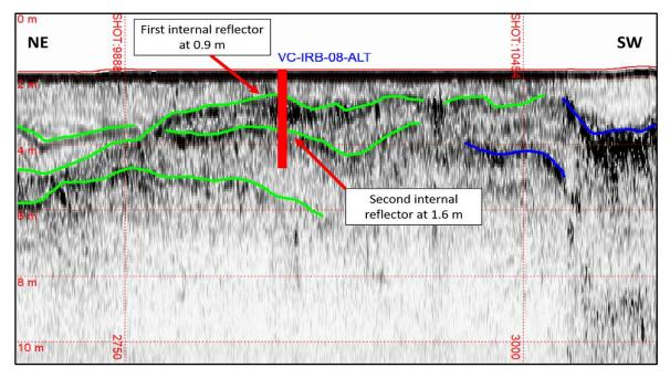
Figure 10.5 Sub-bottom profile showing internal reflectors near core location VC-IRB-08-ALT
