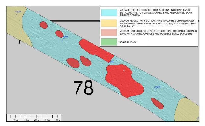
Figure 9.1 Side Scan Sonar Mosaic with Seabed Classification
