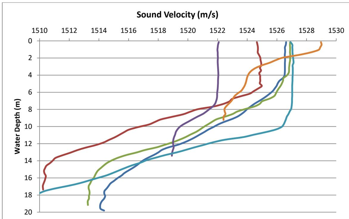
Figure 6.4 Example of SVP profiles collected during the offshore HRG survey
