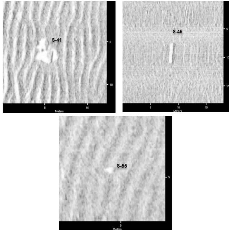
The majority of the seabed along the IR1-Ocean extension is mapped as fine to coarse sand with some gravel (Medium Reflectivity). From KP 21+517 – KP 24+100 a large area is characterized by mixed sediments (silt-clay to sand and gravel; Variable Reflectivity), with significant areas of sand ripple formation. The Variable Reflectivity coincide with seabed areas displaying a more irregular surface in the bathymetry data.
