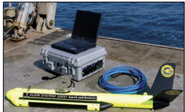
Aboard the RV *Shearwater* the towfish height off seafloor was maintained at 10-20% of the sweep range using a deck mounted hydraulic winch and armored cable. The towfish position was calculated in real-time using the USBL system. A backup positioning system was also used, utilizing a digital cable counter sheave to measure cable out from the stern of the vessel.
