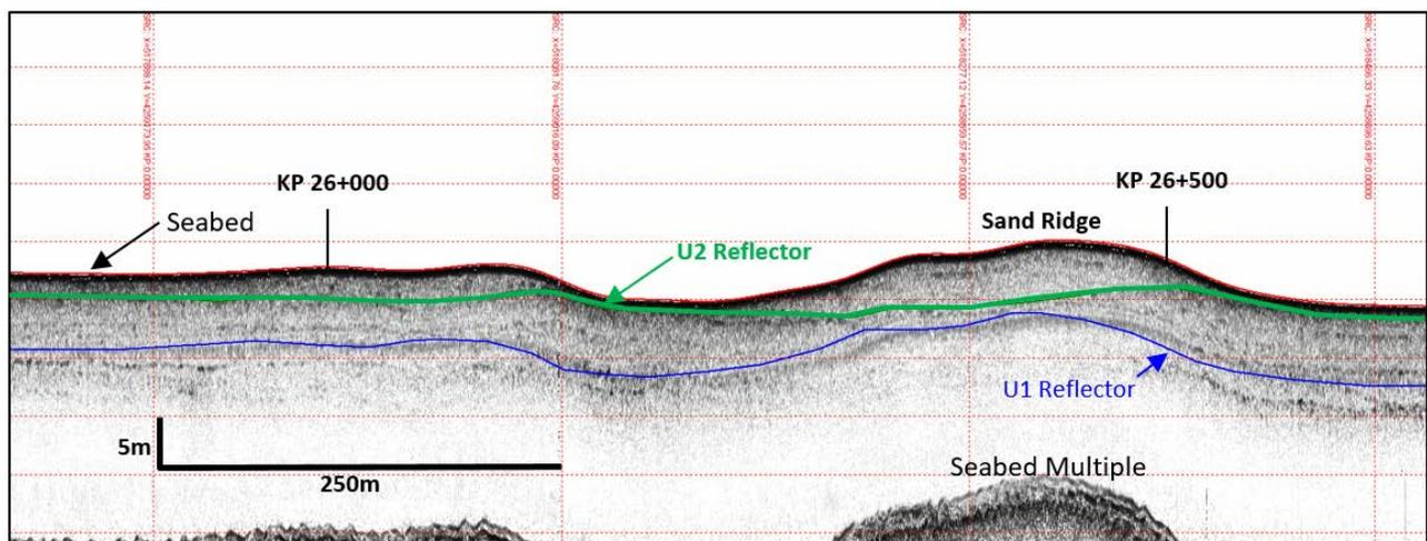
Figure 9.15 Sub-bottom Profile showing Sand Ridge
