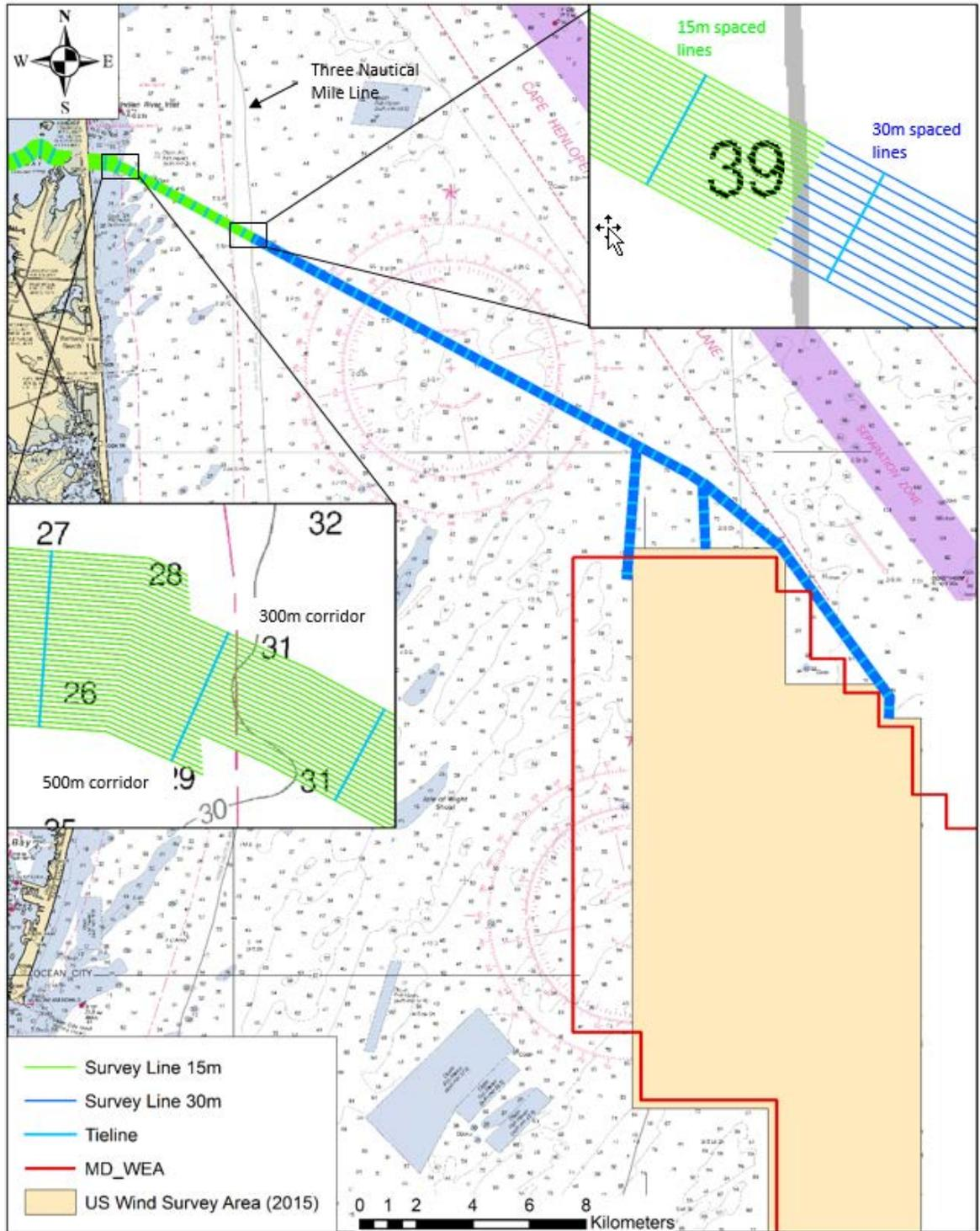
Figure 6.1 Offshore export cable survey line plan
