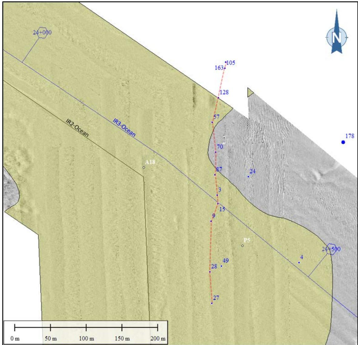
Figure 9.13 Linear Arrangement of Magnetic Anomalies near KP 24+300
