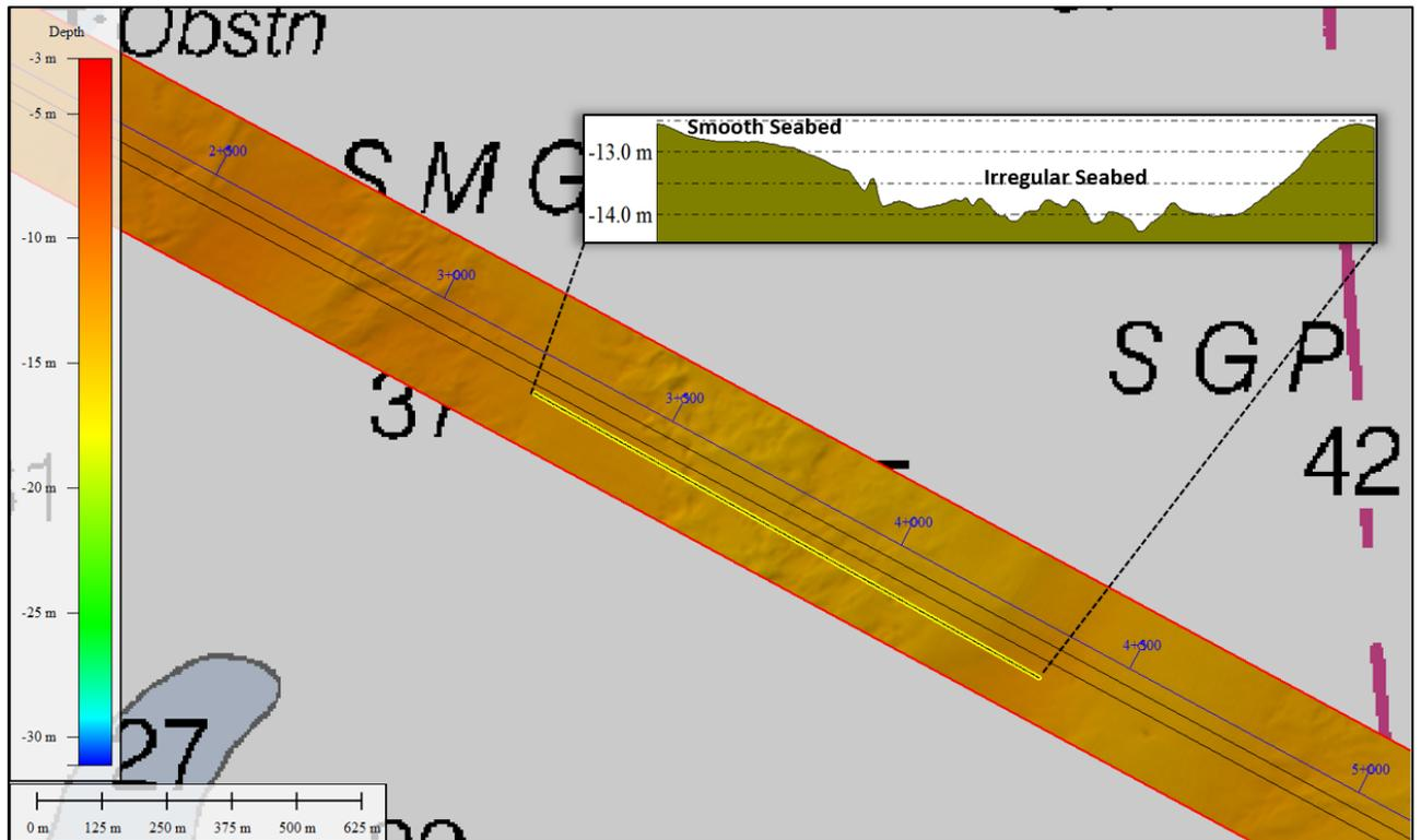
Figure 9.4 Bathymetry between KP 3+000 – 4+500 Showing Transition From Smooth to Irregular Bottom
