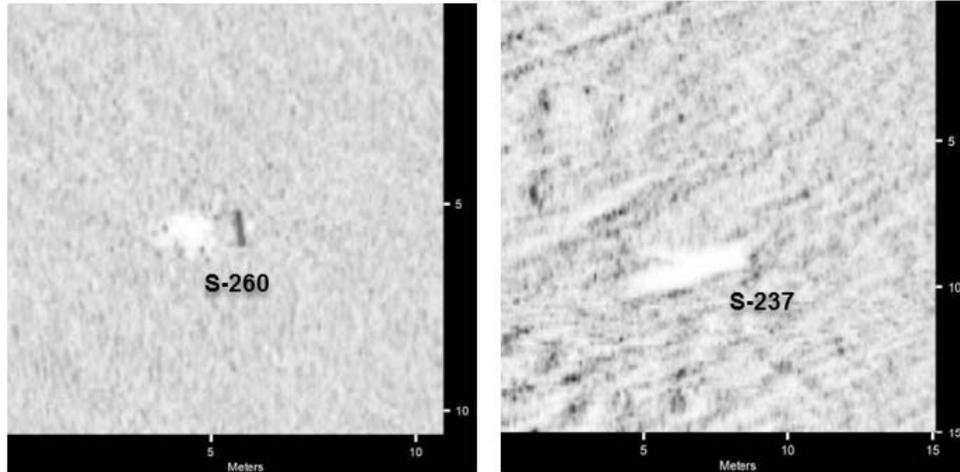
The seabed between KP 18+000 – 22+000 is predominantly fine to coarse sand with some gravel (Medium Reflectivity). From KP 22+000 – 24+500 the bottom is characterized by mixed sediments (silt-clay to sand and gravel; Variable Reflectivity), with several areas of Medium-High Reflectivity (coarse sand, gravel, cobbles and possible boulders). The Variable Reflectivity areas again correlate to the irregular seabed areas as seen in the bathymetry data.
