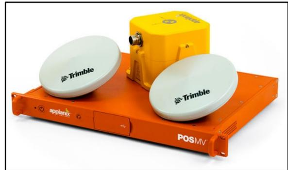
Aboard the RV *Shearwater* the IMU was mounted on the floor of the survey laboratory near the vessel's center of rotation/gravity. The GPS antennas were mounted above ship's bridge roof, aligned normal to the longitudinal axis of the vessel. Offsets between the GPS antennas, IMU and all other fixed mounting points for the other geophysical sensors were precisely measured before conducting onsite calibrations.
