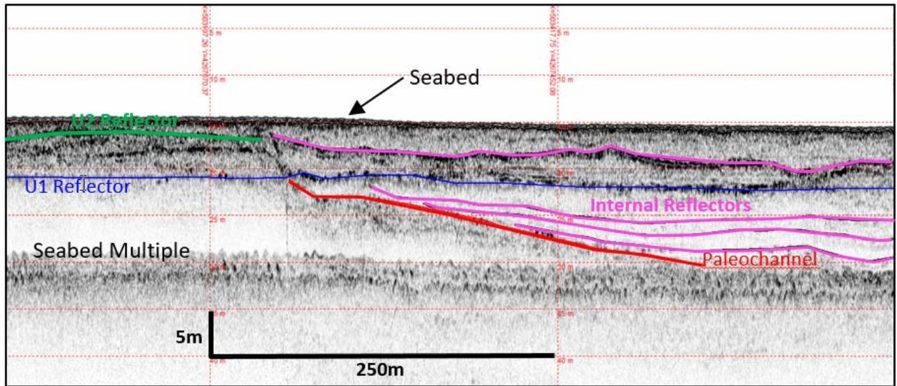
Figure 9.10 Northwest Flank of Paleochannel near KP 9+000
