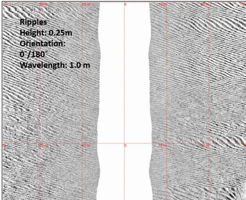
Figure 9.6 Sand Ripples between KP 0+000 – 0+500
