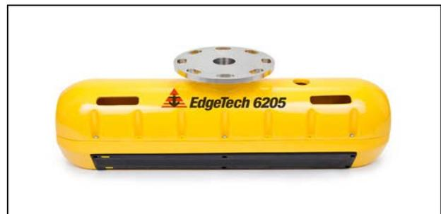
The Edgetech 6205 is particularly useful in shallow settings such as Indian River Bay, because the system can acquire larger swath coverage than most conventional MBES. In addition to greater efficiency, the collection of side scan sonar within the same system eliminates positioning errors that are common when surveying in shallow locations.
