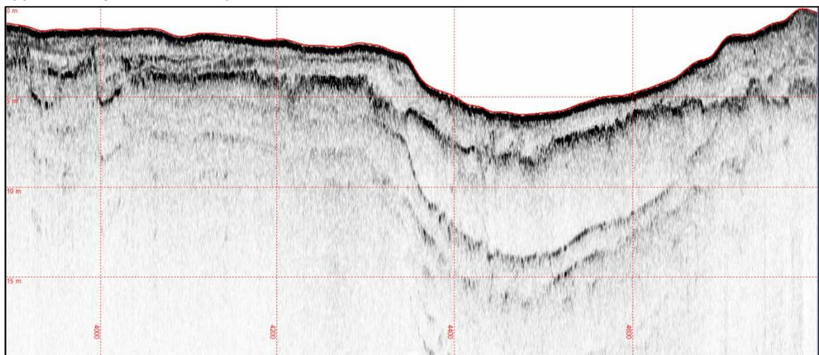
Figure 6.7 Edgetech 3100P data example showing seafloor penetration
