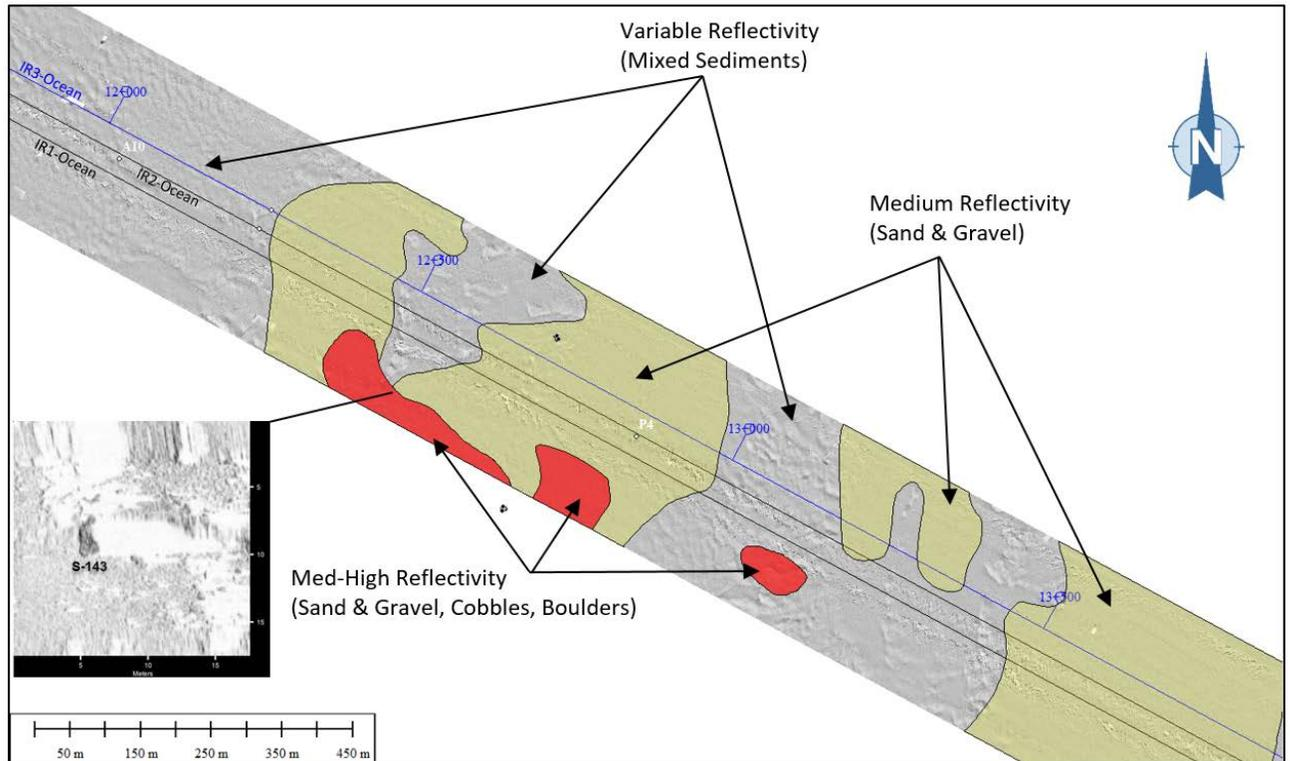
Figure 9.9 Side Scan Sonar Mosaic with Seabed Classification, KP 12+000 – 13+800
