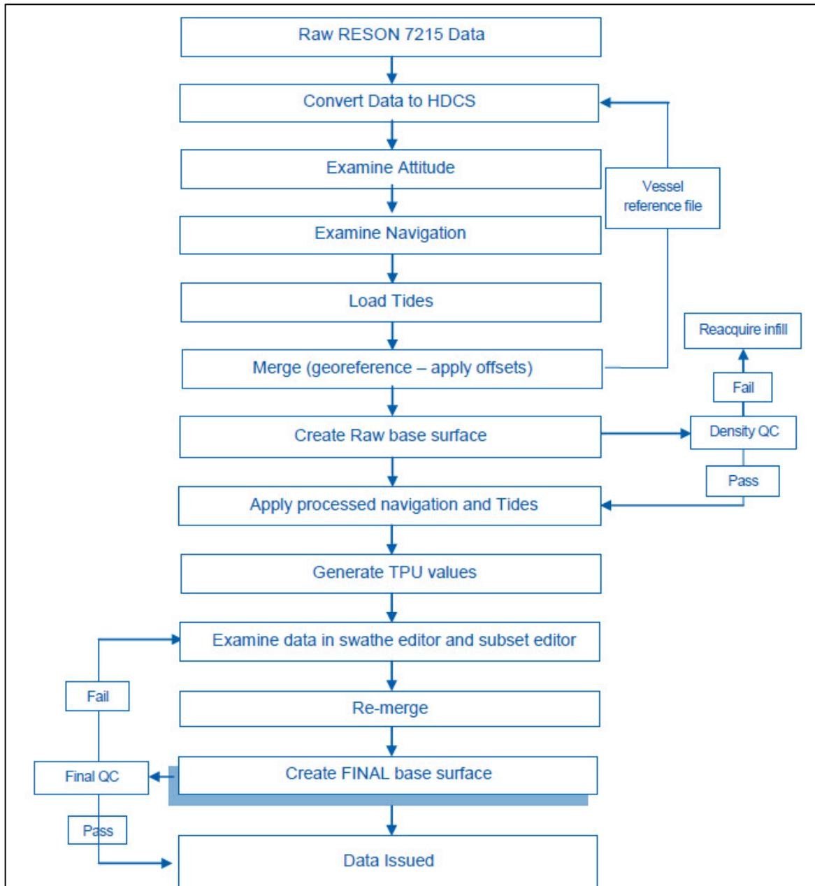
Figure 8.1 MBES processing flow diagram for bathymetry data
