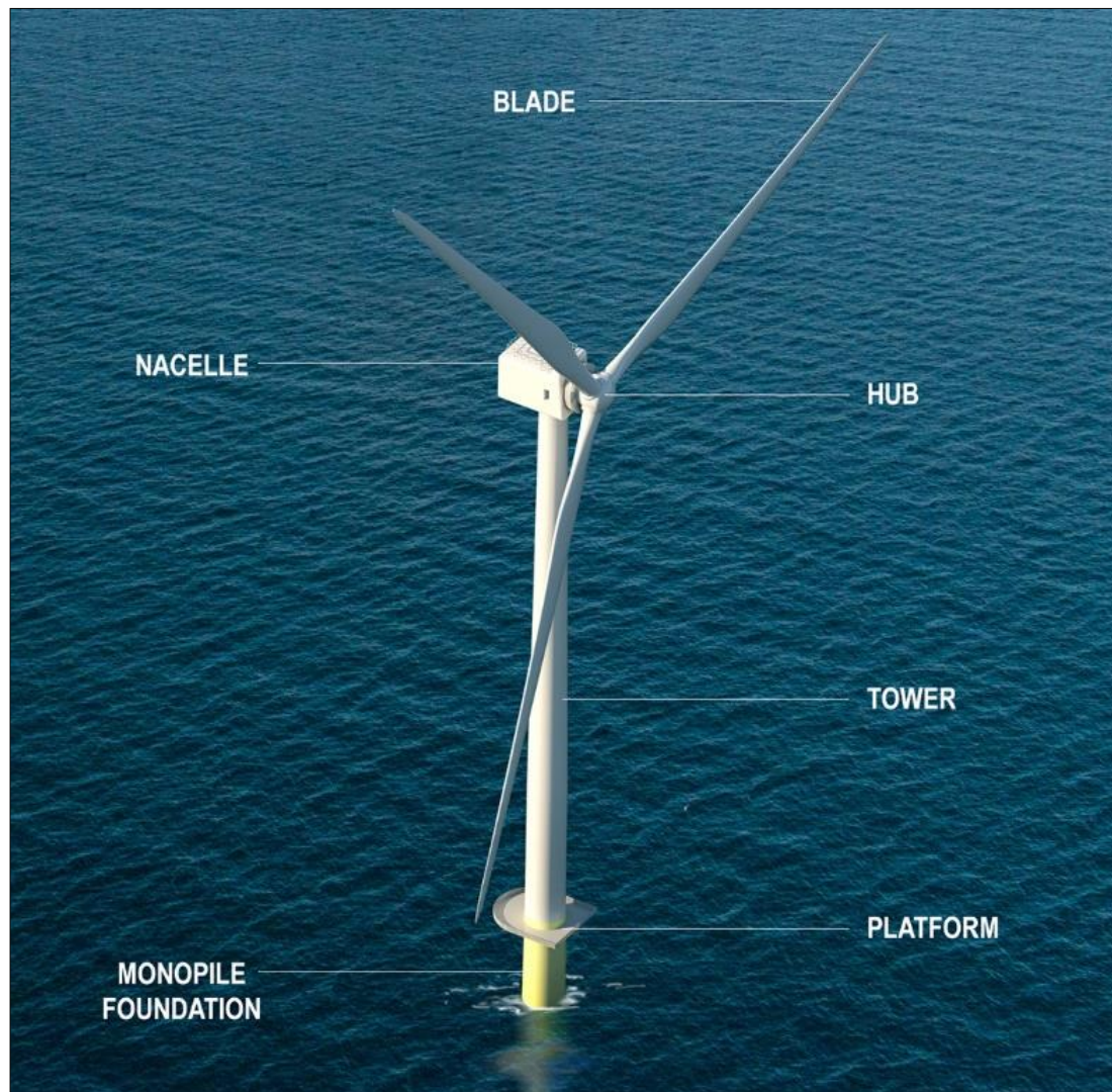
Inset 1.1-3 – Diagram of the Wind Turbine Generator Components
