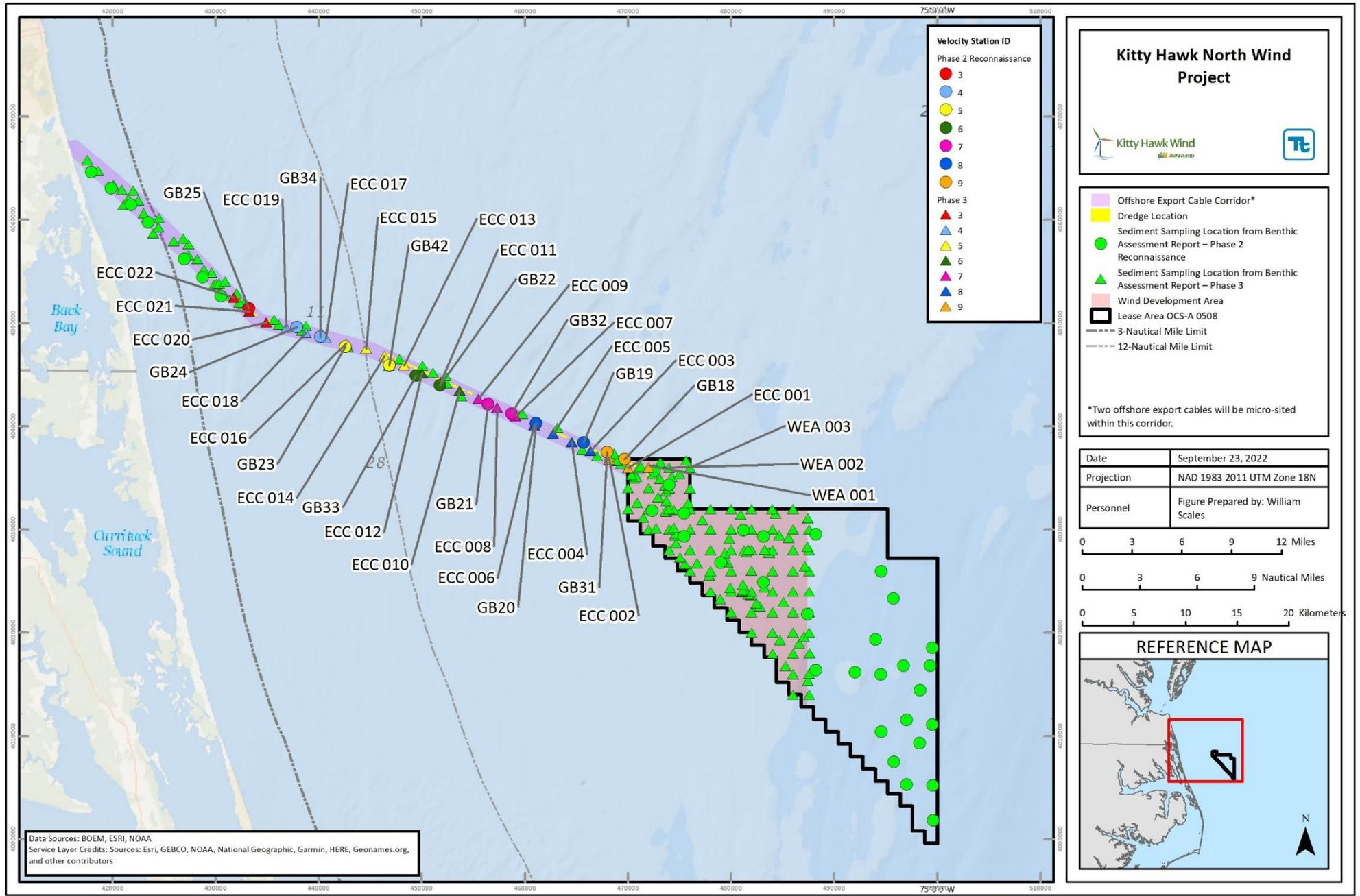
Figure M-4 Sediment Sampling Locations used for Sediment Transport Analysis of Pre-Cable Installation Dredging
