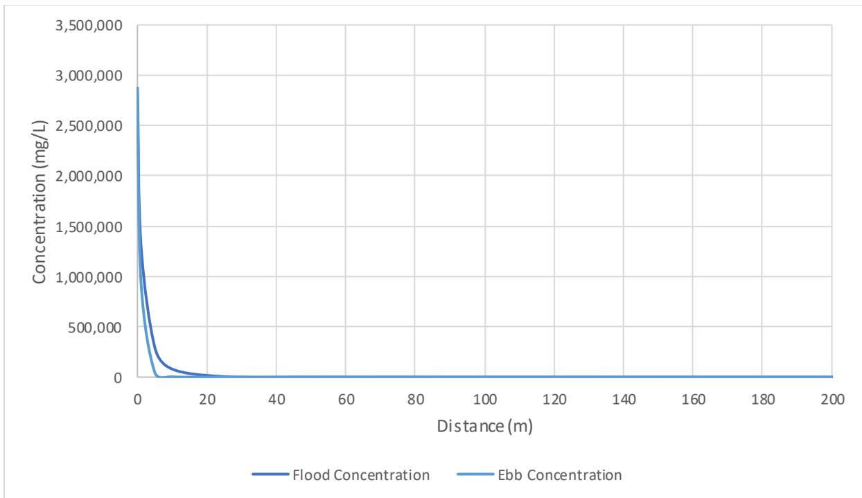
**Figure M-9 Maximum Flood and Ebb Tide Suspended Sediment Concentrations at GB19 (88% fine sediment)**
