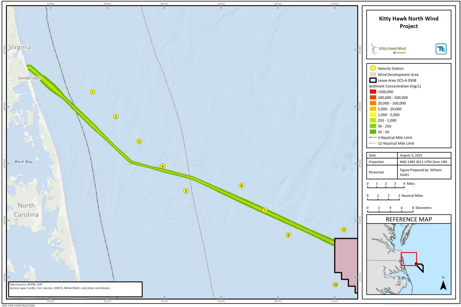
**Figure M-11 Maximum Flood Tide Suspended Sediment Concentrations along the Offshore Export Cable Corridor**
