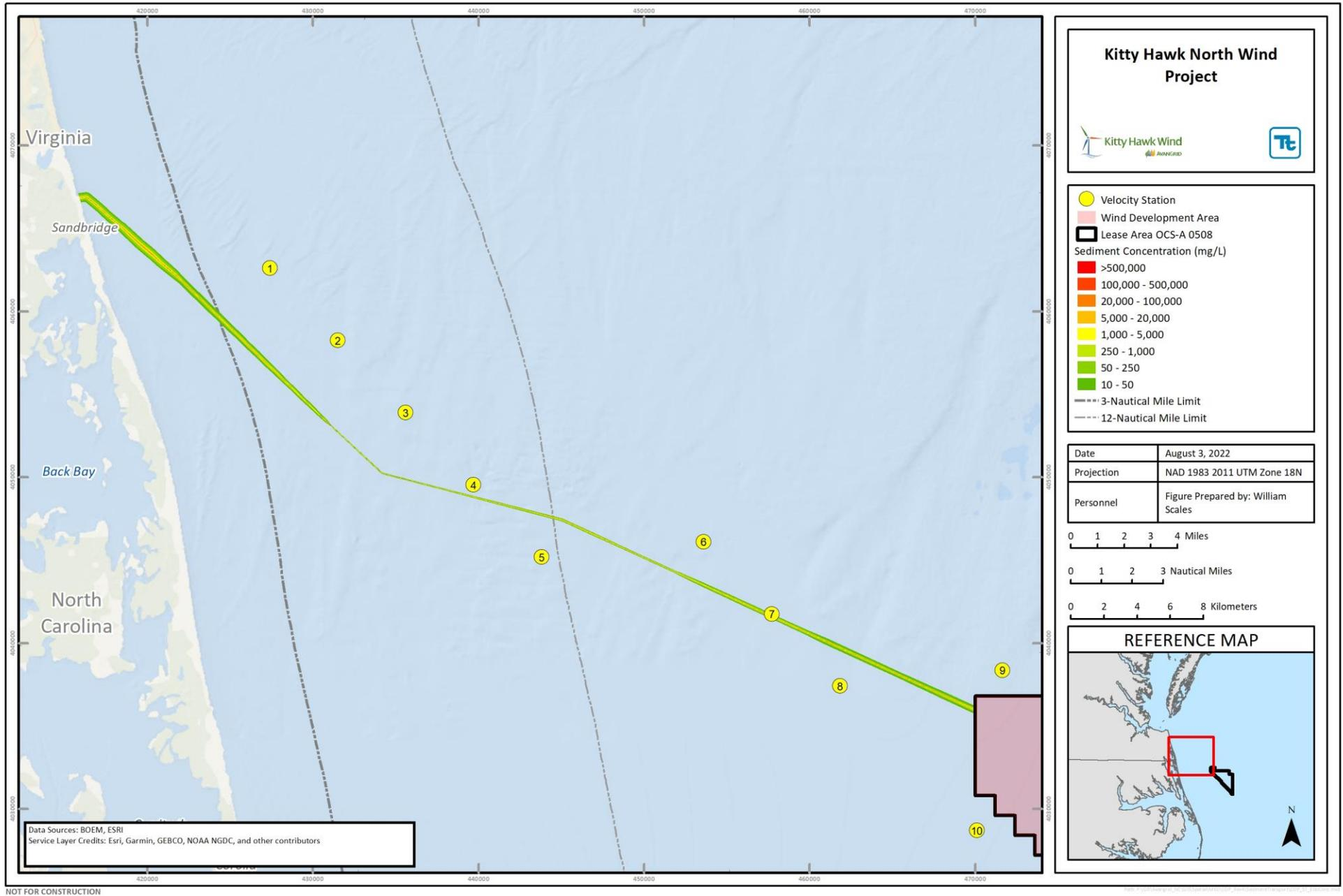
**Figure M-12 Maximum Ebb Tide Suspended Sediment Concentrations along the Offshore Export Cable Corridor**
