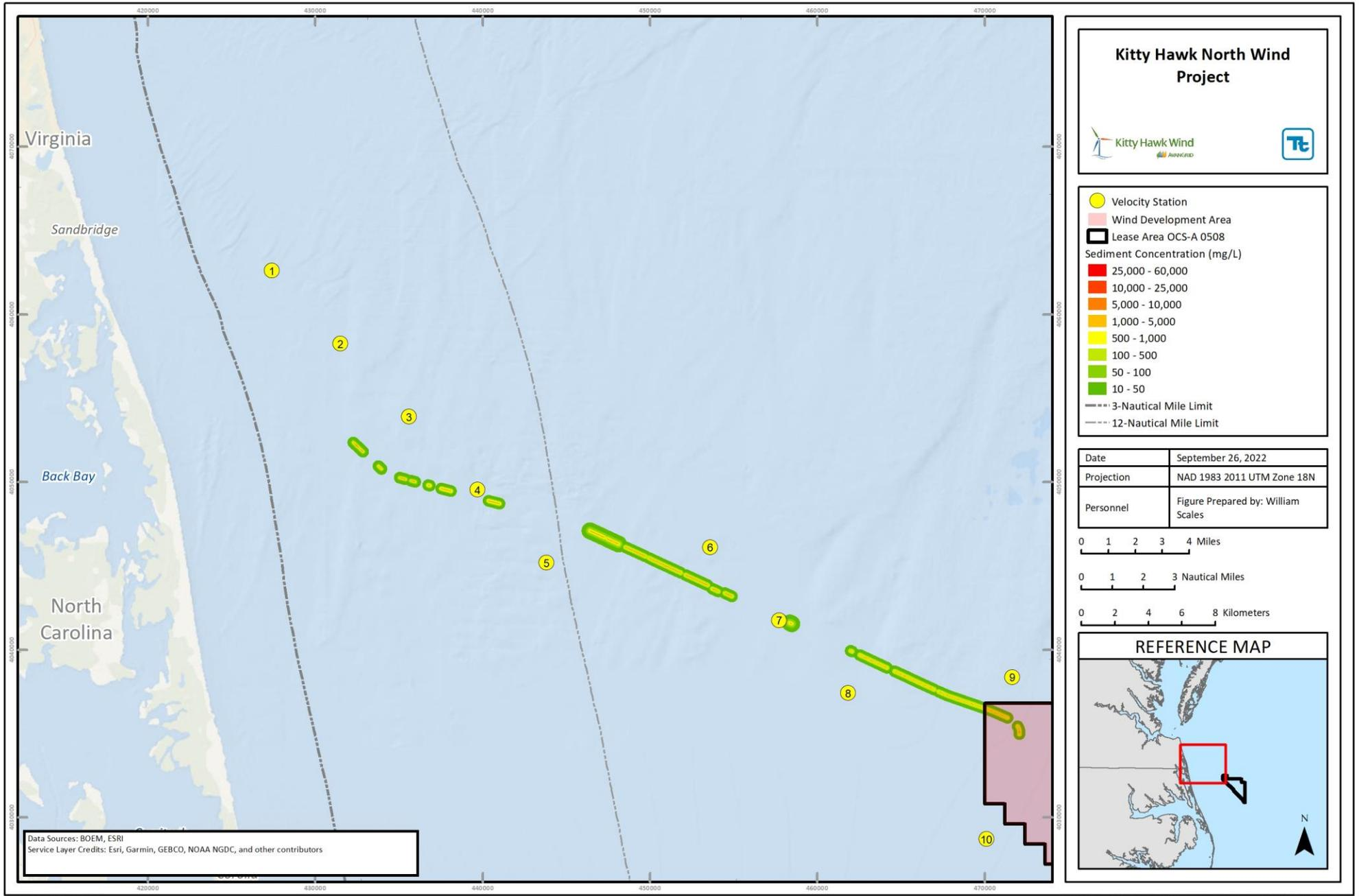
Figure M-5 Maximum Flood Tide Suspended Sediment Concentrations from Hopper Overflow during Dredging
