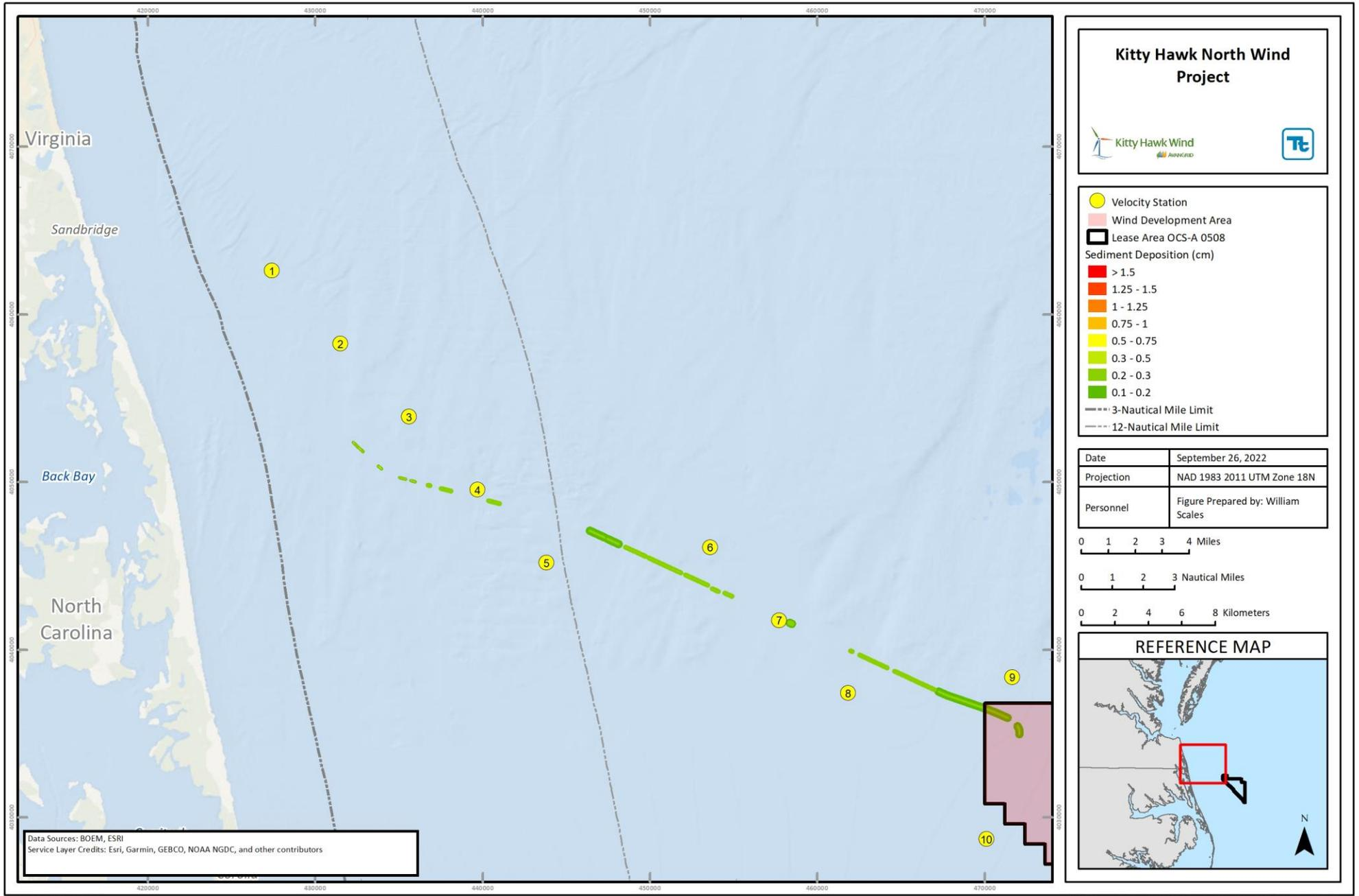
Figure M-7 Maximum Flood Tide Sediment Deposition from Hopper Overflow during Dredging
