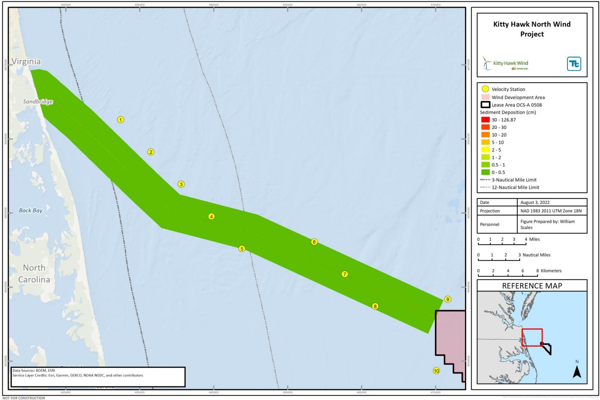
**Figure M-14 Maximum Ebb Tide Sediment Deposition along the Offshore Export Cable Corridor**
