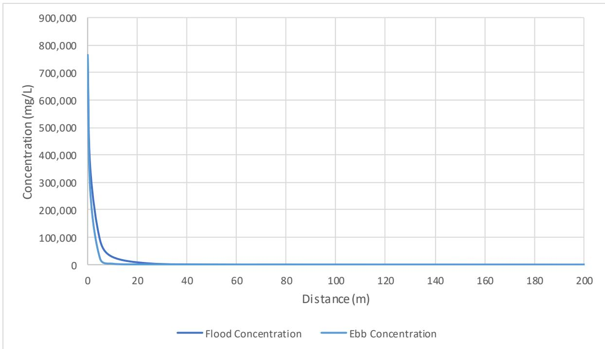
**Figure M-10 Maximum Flood and Ebb Tide Suspended Sediment Concentrations at GB38 (24% fine sediment)**
