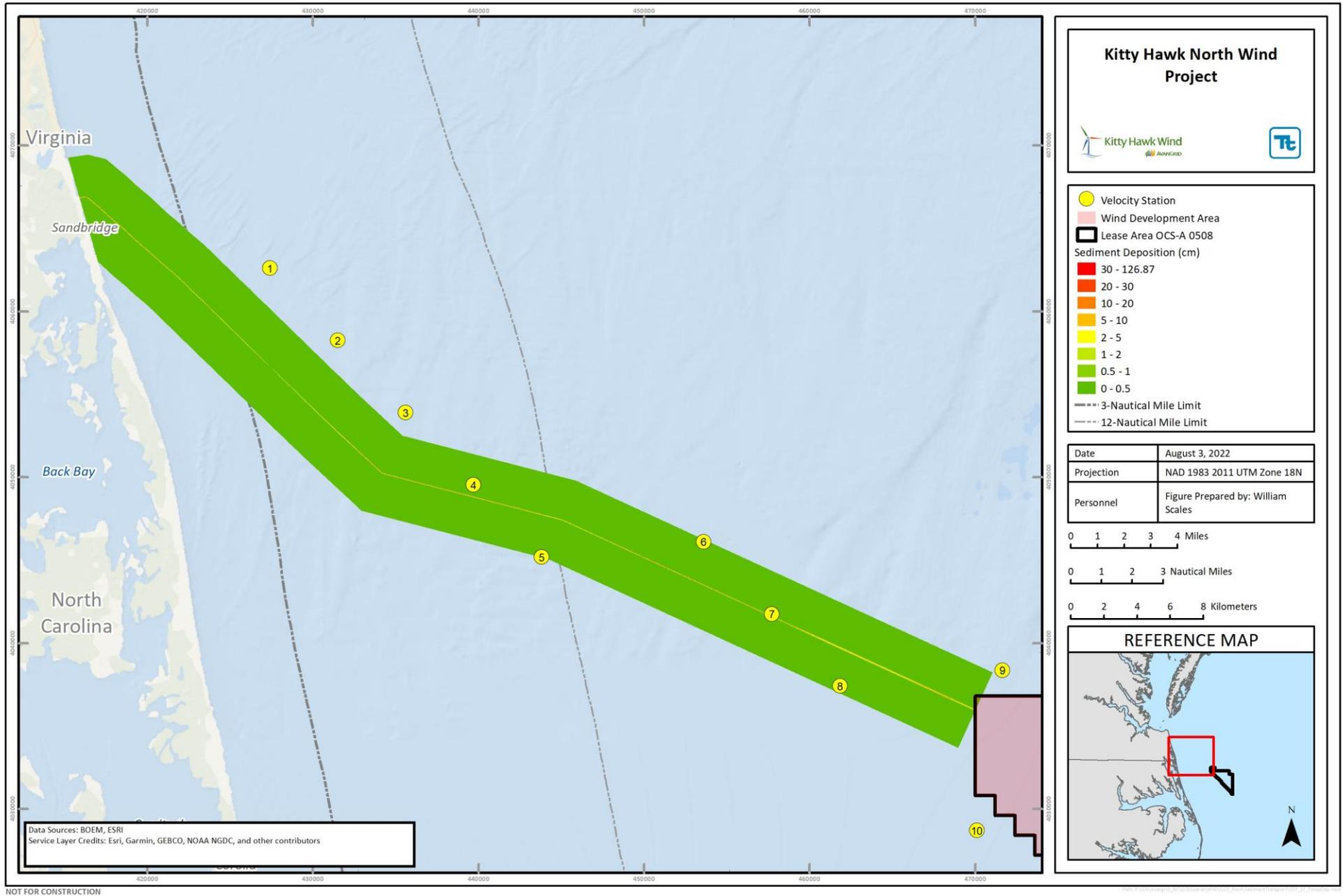
**Figure M-13 Maximum Flood Tide Sediment Deposition along the Offshore Export Cable Corridor**
