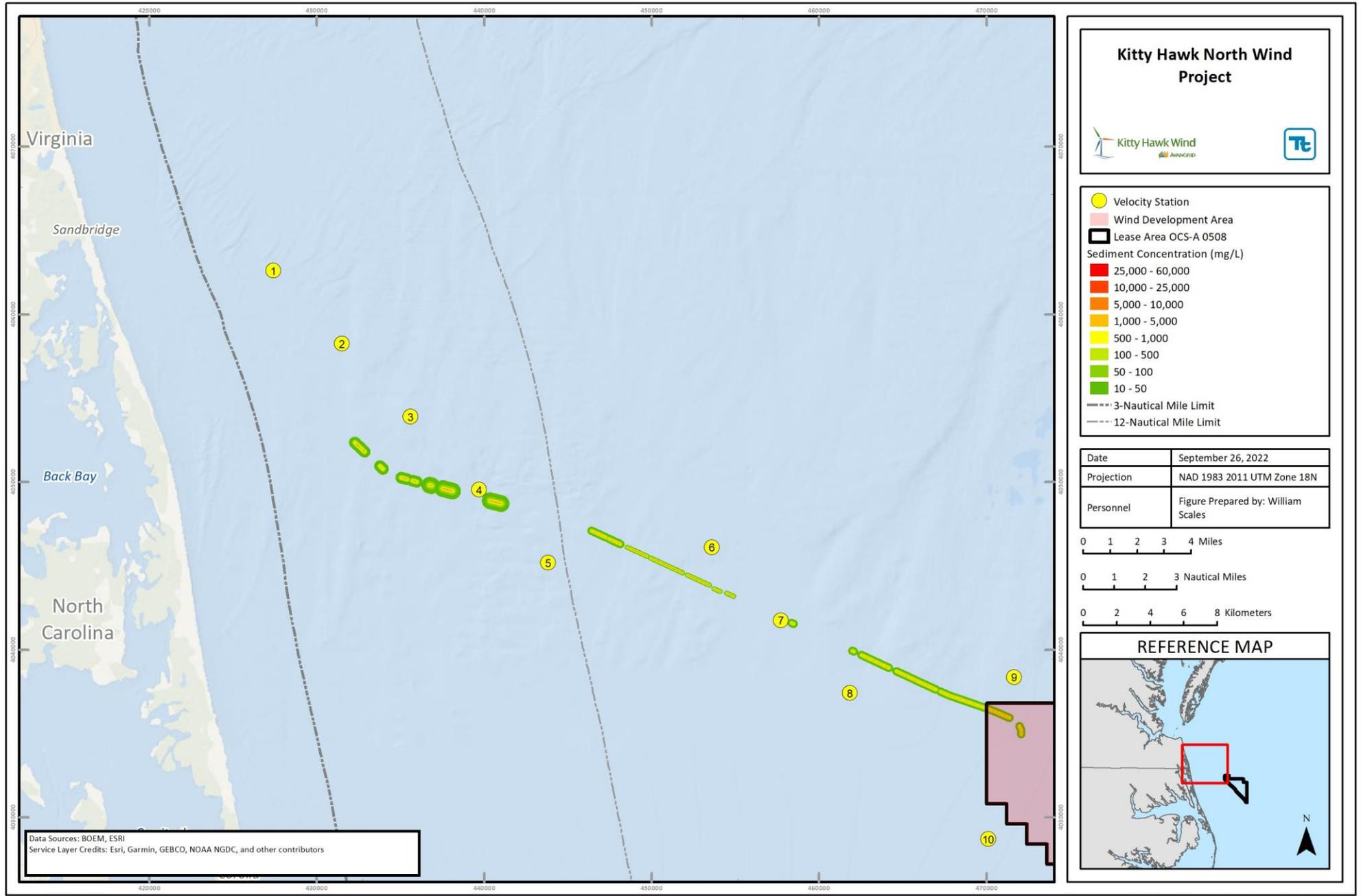
Figure M-6 Maximum Ebb Tide Suspended Sediment Concentrations from Hopper Overflow during Dredging
