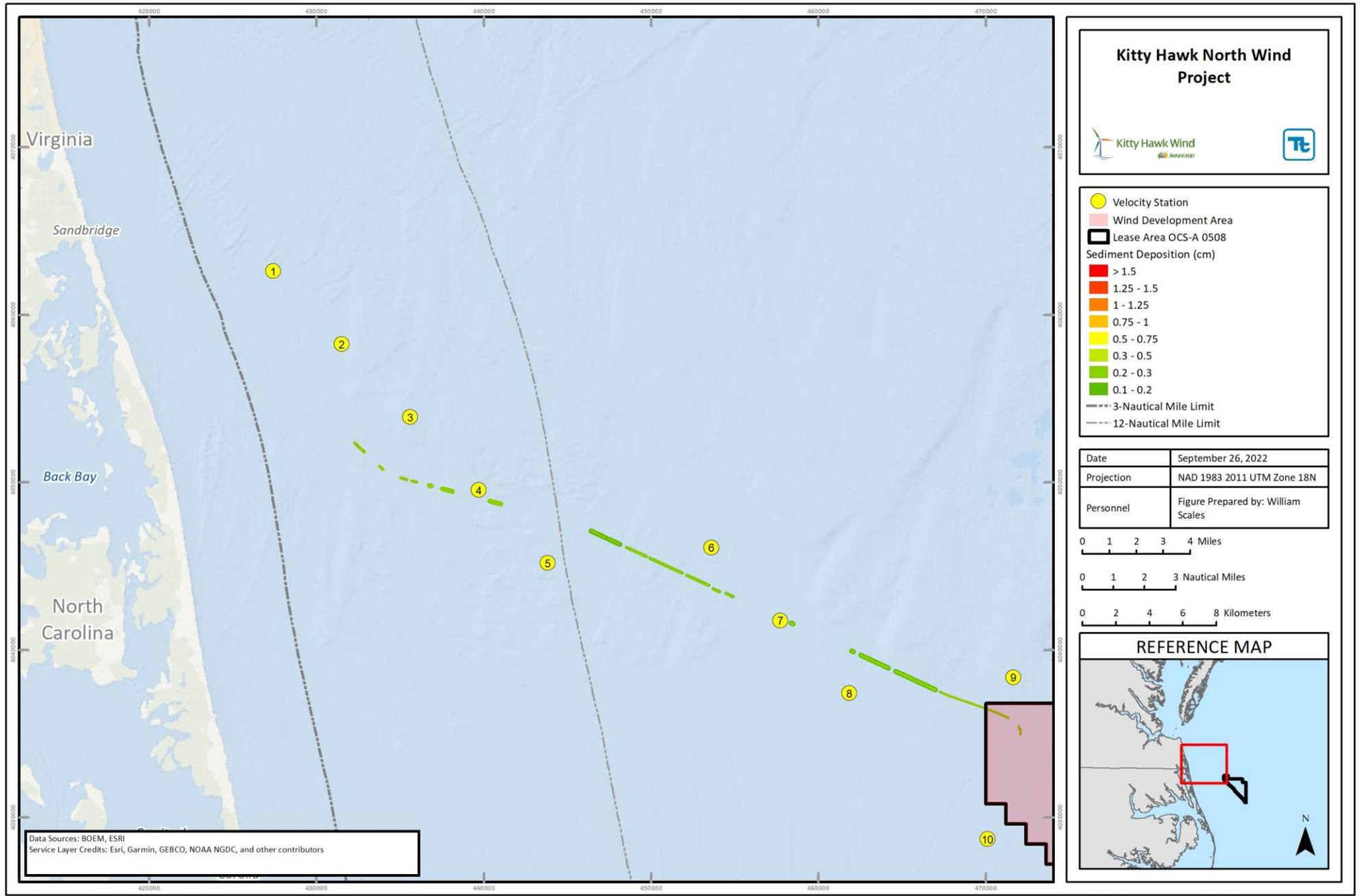
Figure M-8 Maximum Ebb Tide Sediment Deposition from Hopper Overflow during Dredging
