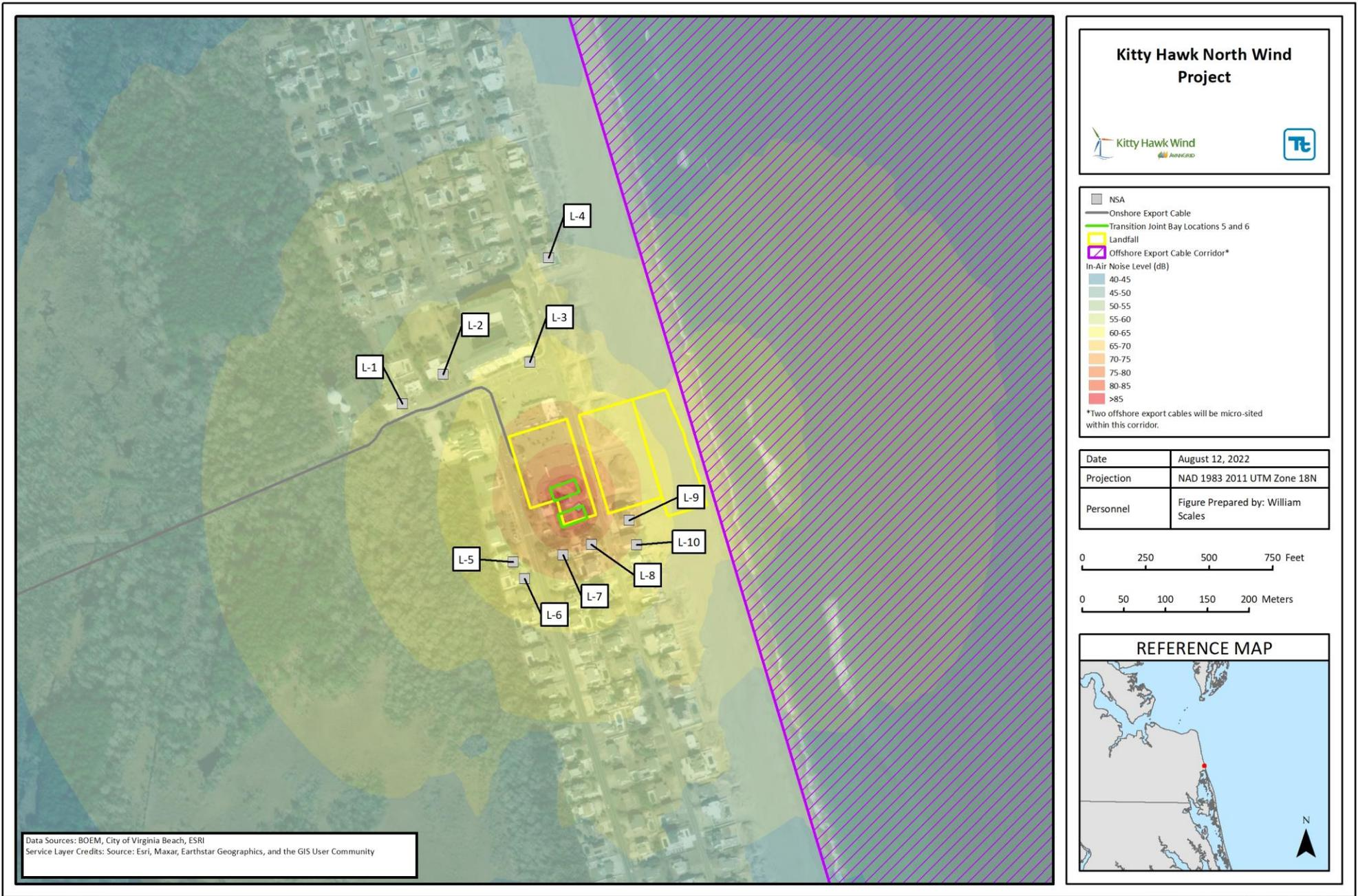
Figure O-5. HDD 5 and HDD 6 Contour Isopleth
