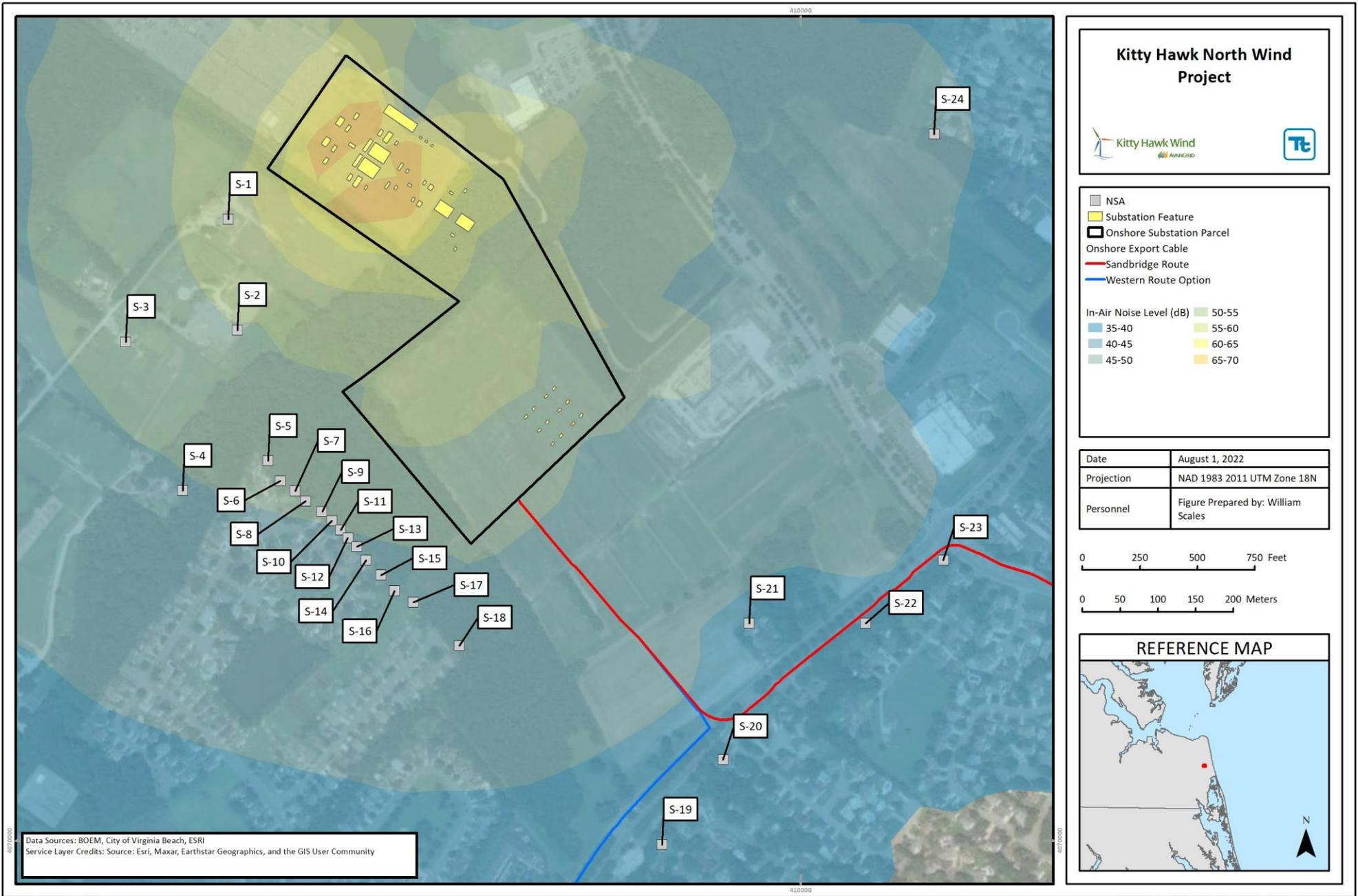
Figure O-8. Onshore Substation Site Operational Sound Levels
