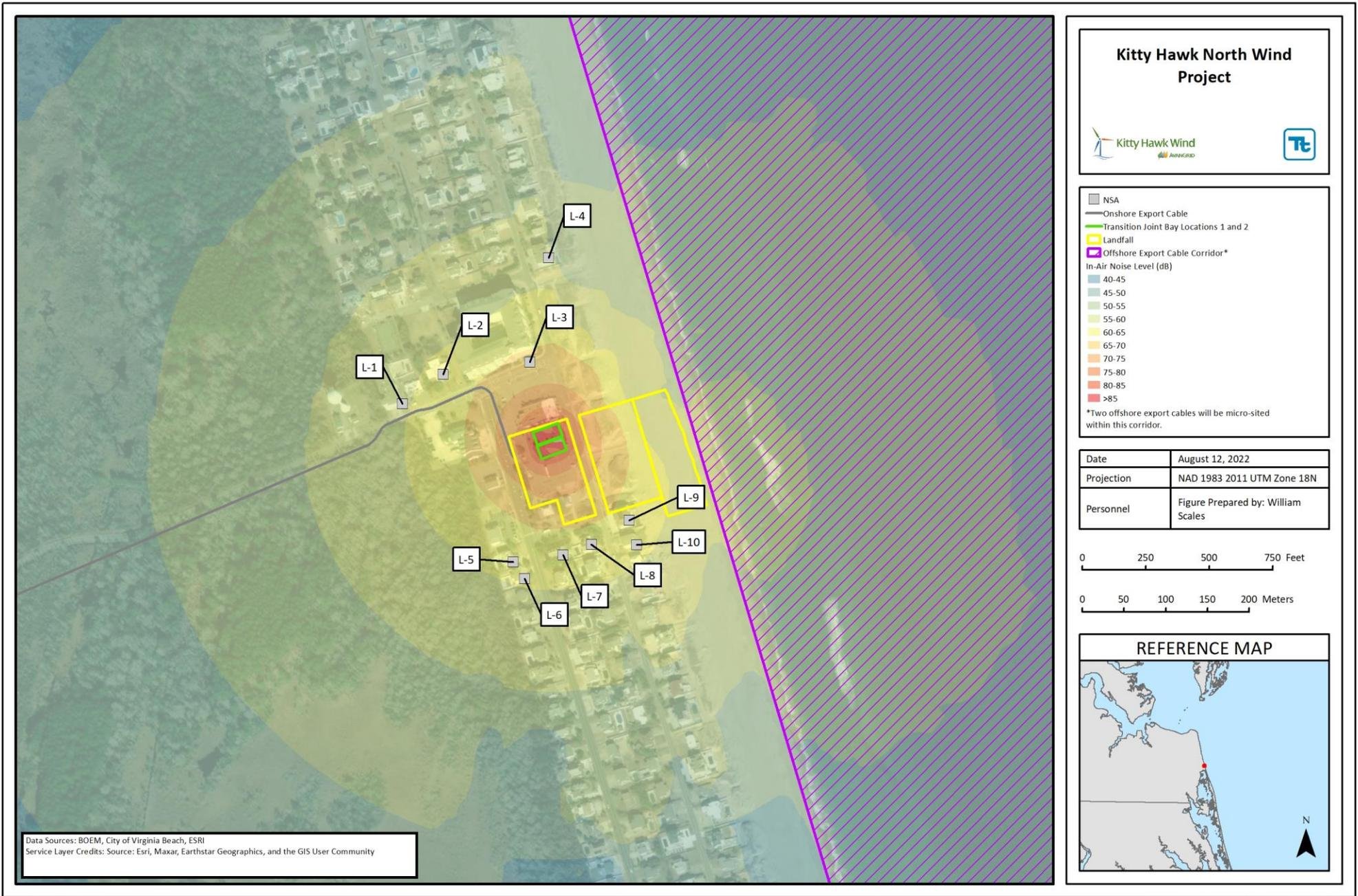
Figure O-3. HDD 1 and HDD 2 Contour Isopleth
