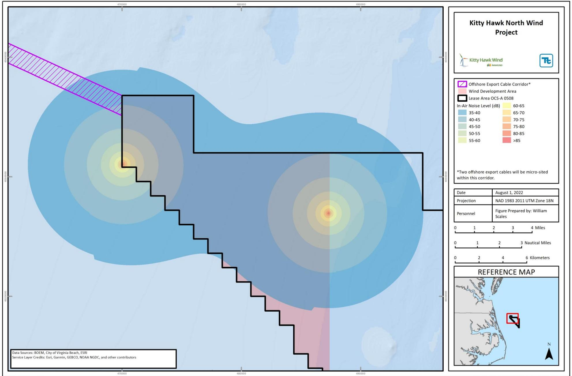
Figure O-6. Impact Pile Driving Received Sound Levels (In-Air)
