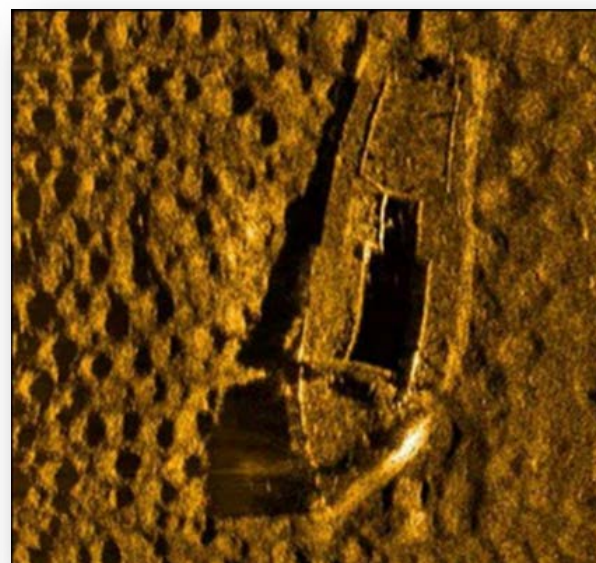
Image of the EdgeTech 4200 Sidescan Sonar towfish (left) and data example depicting a shipwreck and adjacent seafloor from the northern Gulf of Mexico, offshore Louisiana in approximately 35 ft of water depth (right).
