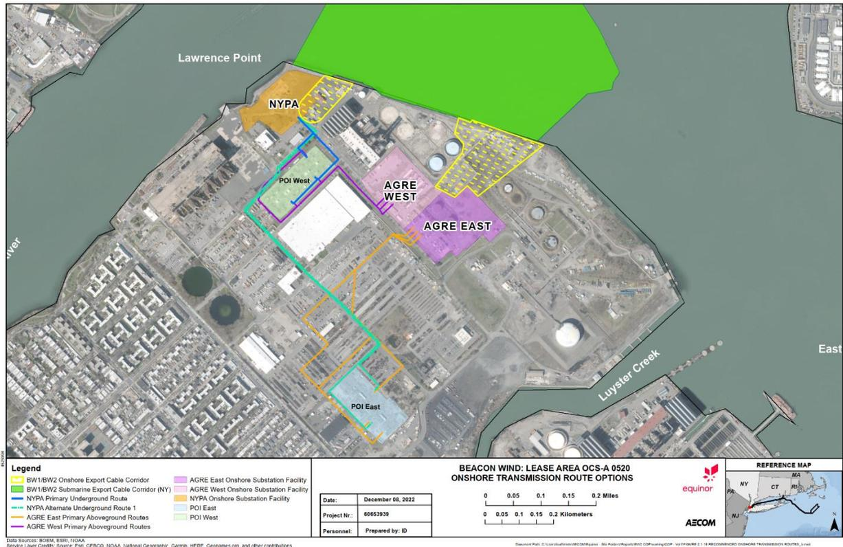
**Figure 2. Depiction of the Astoria Power Complex for the BW1 Onshore Electric Transmission System with the Proposed Converter Station Facility Locations, the Location of the HVDC Onshore Export Cables, and the HVAC Onshore Interconnection Cables.**
