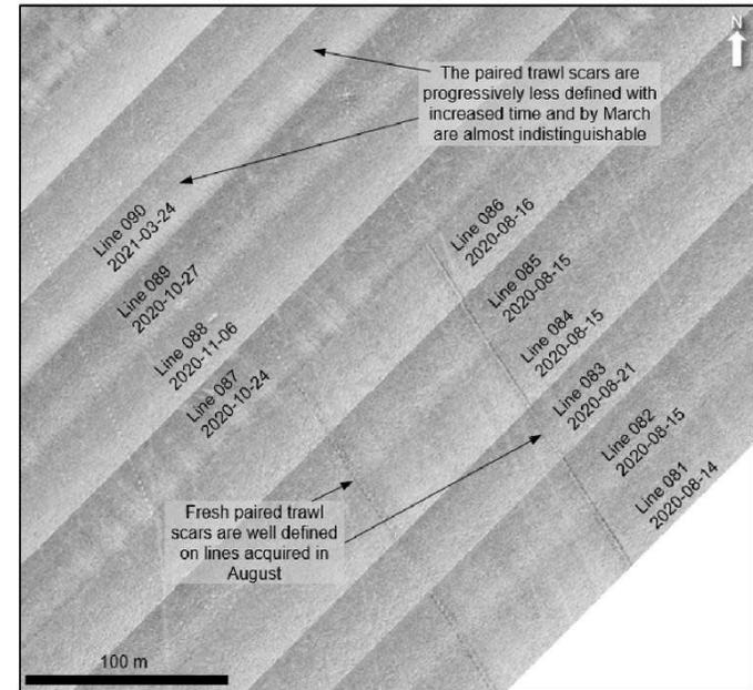
Figure EE.3-4.b Side-scan sonar imagery showing the dissolution of a paired trawl scar through time within the lease area.
