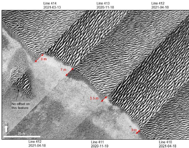
Figure EE.3-4.a Side-scan sonar imagery showing time-variant offset along the edge of a sorted bedform within the lease area.
