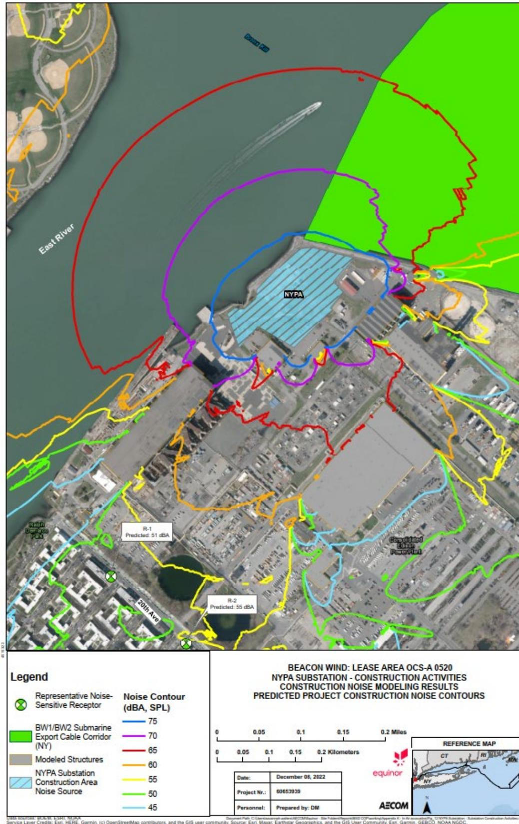
**FIGURE K.5-12. PREDICTED NOISE CONTOURS FOR COMBINED SUBSTATION CONSTRUCTION ACTIVITIES AT NYPA AND AGRE EAST**
