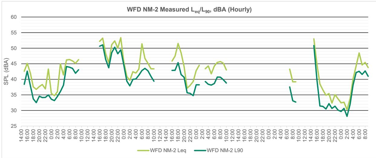
Note: Gaps in measured SPL represent periods where data suggest the connection between the sound level meter and microphone were interrupted or disconnected due to unknown factors.
