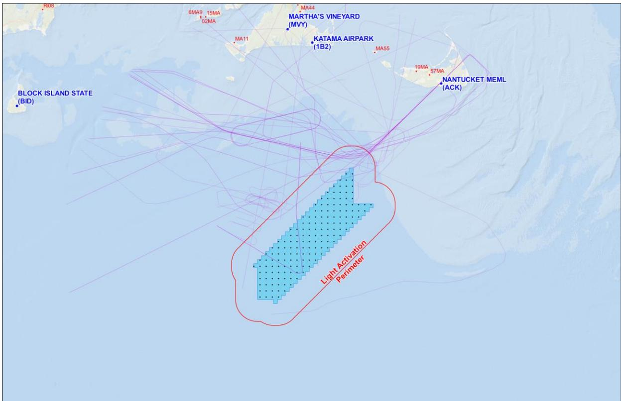
**Figure 3: Flight tracks (purple) that would have activated ADLS obstruction lights (based on 1,116-foot tall (340.2 meter) wind turbines and 2019 FAA NOP data)**
