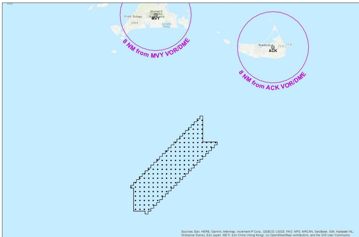
**Figure 12: NAVAID protection areas in proximity to the Beacon Wind project**
