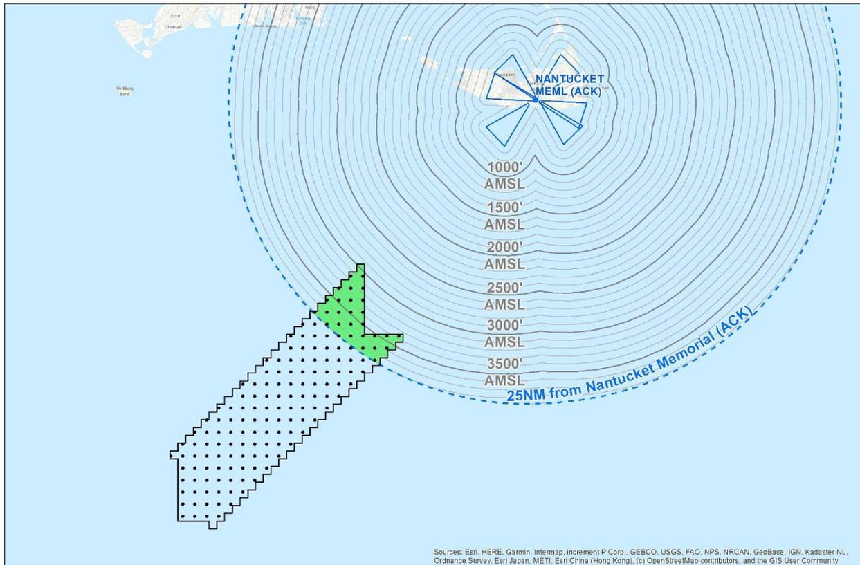
**Figure 6: Nantucket Memorial (ACK) obstacle departure procedure assessment**
