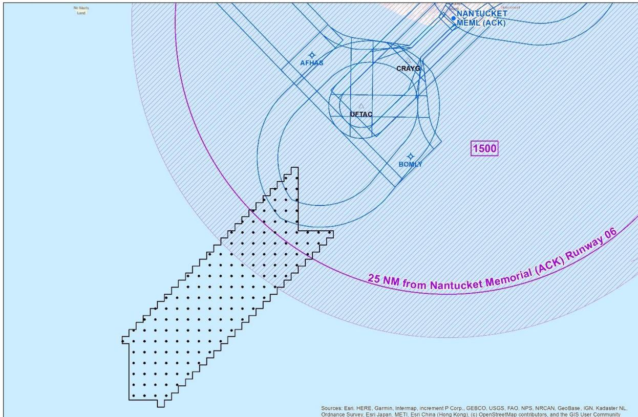
**Figure 7: Nantucket Memorial (ACK) RNAV (GPS) Approach to Runway 06 (blue) with MSA obstacle evaluation area (hatched purple)**
