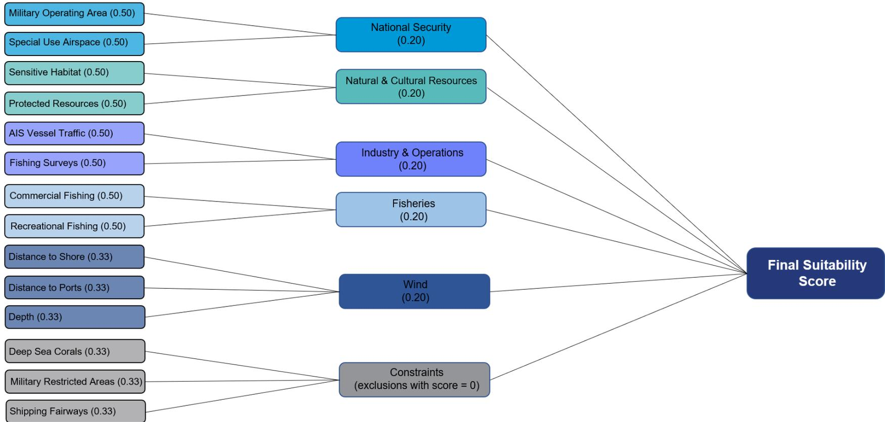
**Figure 2.6.** A generalized approach to a Multi-Criteria Decision Analysis suitability model with equally-weighted data layers in the submodels and final suitability model. Note that not all of the data layers are shown.
