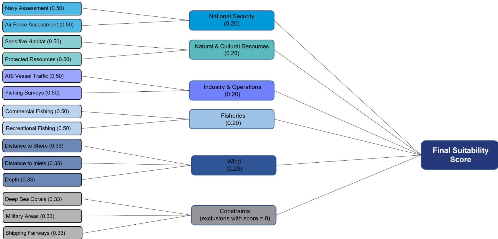
**Figure 2.6.** A generalized approach to a Multi-Criteria Decision Analysis (MCDA) suitability model with equally-weighted data layers in the submodels and final suitability model. Note that not all of the data layers are shown.
