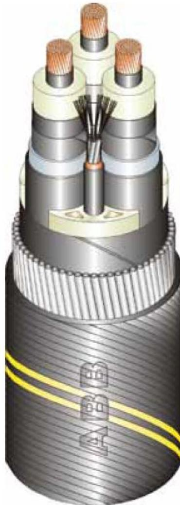
**Figure 3.3-9. Cross-Section of Typical Subsea Cable**
