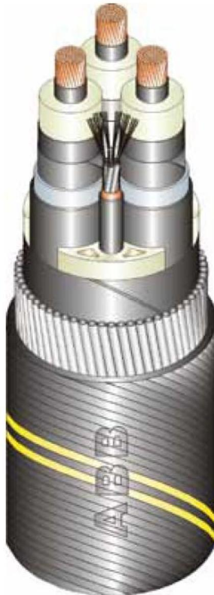
**Figure 3.3-5. Representative Cross Section of an Inter-Array Cable**
