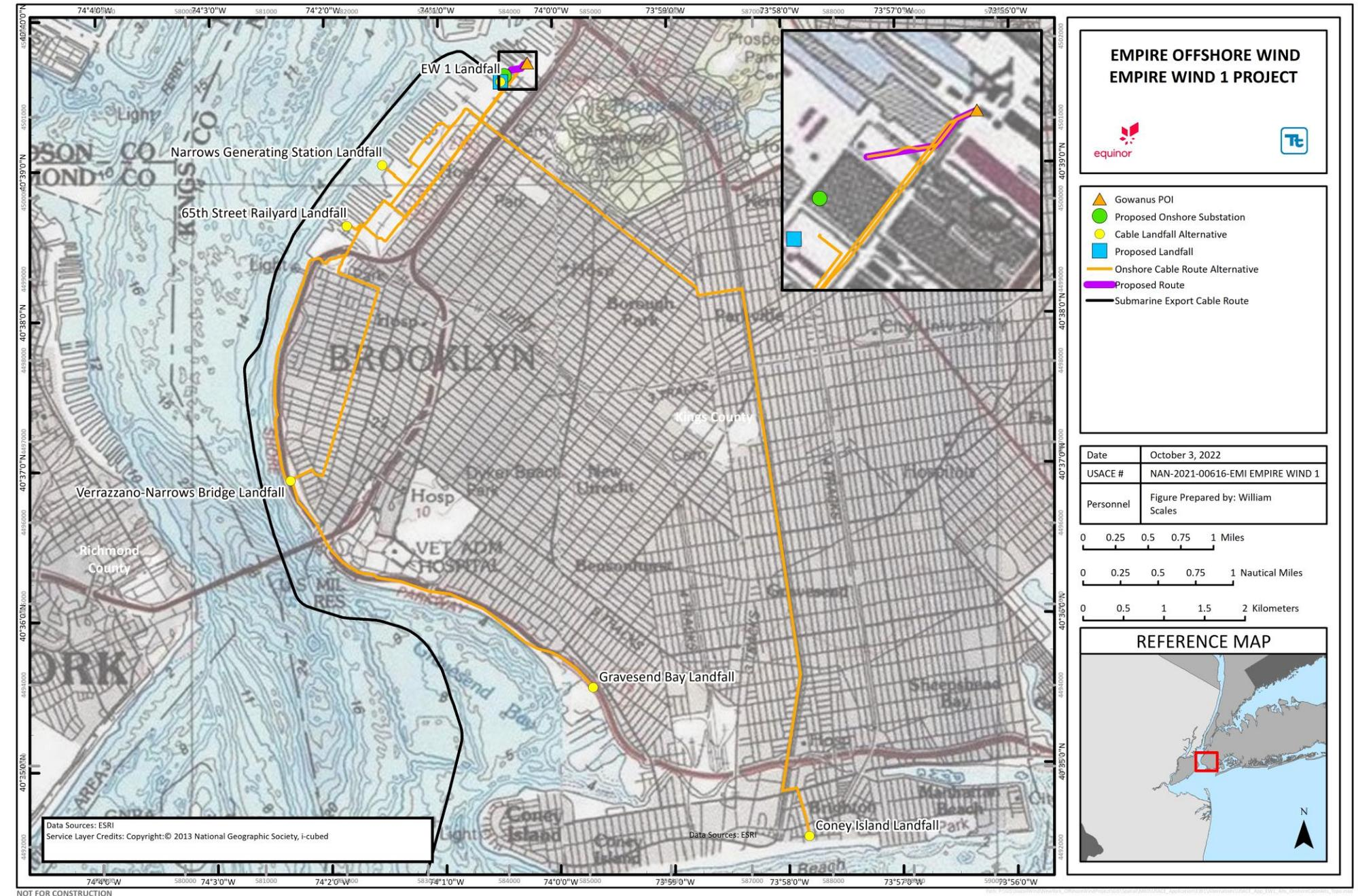
**Figure 3 Cable Landfall and Onshore Cable Route Alternatives**
