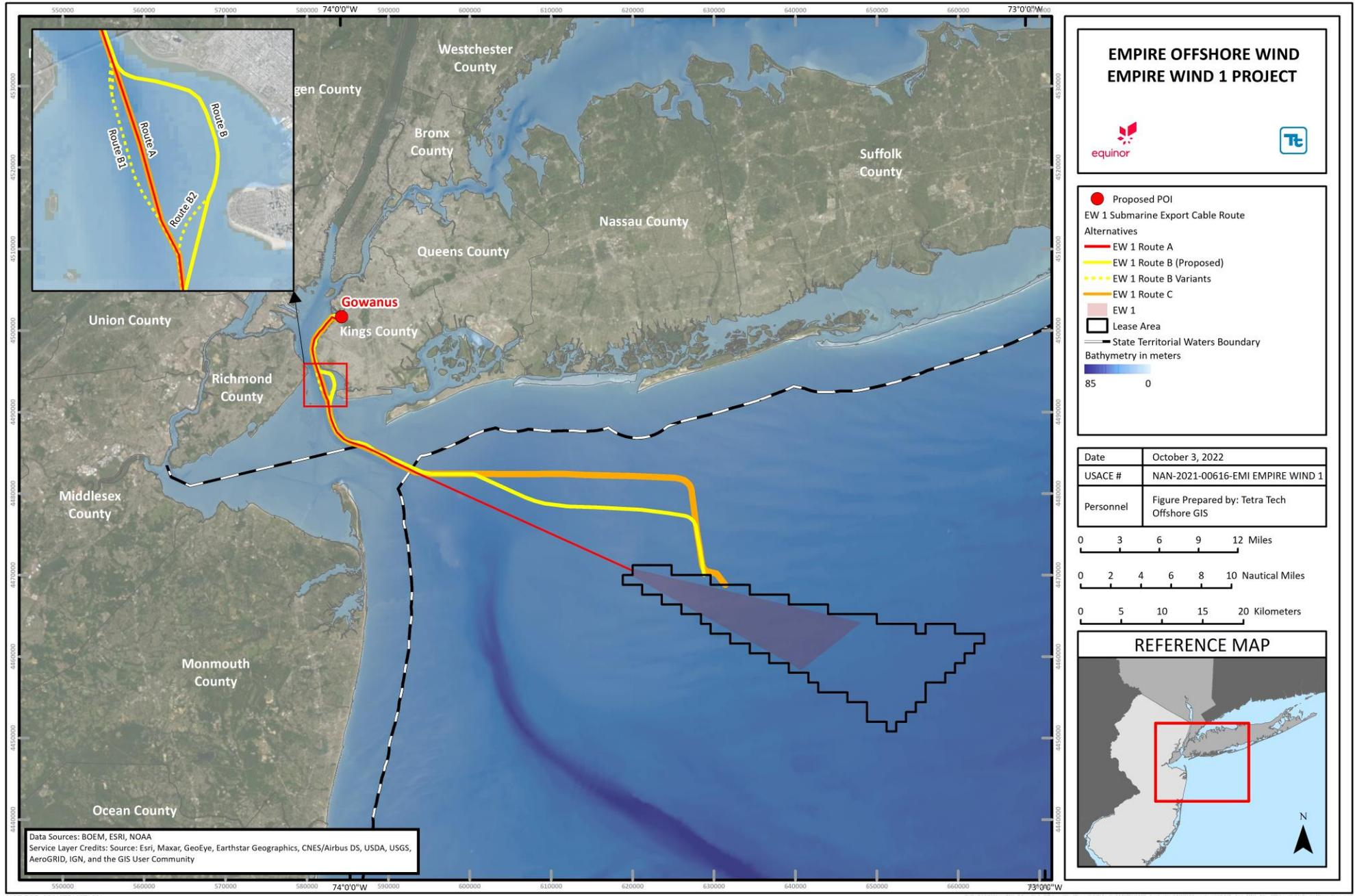
Figure 1 Submarine Export Cable Route Alternatives – Federal Waters
