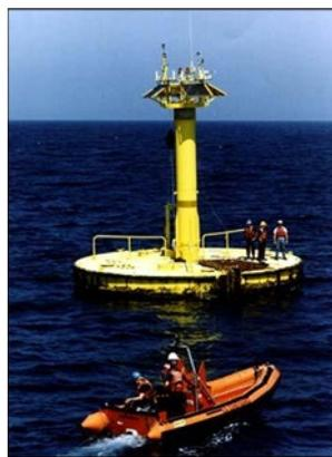
**Figure 4: 10-Meter Discus-Shaped Hull Buoy**
