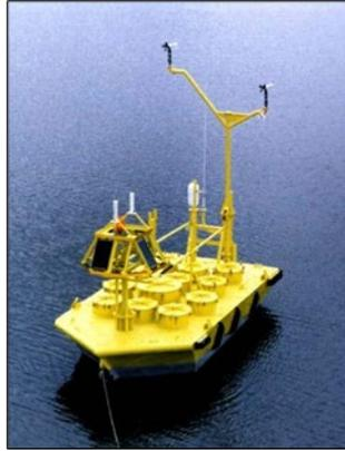
**Figure 5: 6-Meter Boat-Shaped Hull Buoy**
