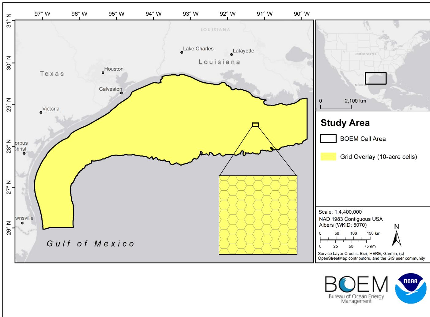
Figure 2.3. An example of the grid cells formulated for the Call Area. Each cell is a 10-acre or 4.05-ha hexagon.
