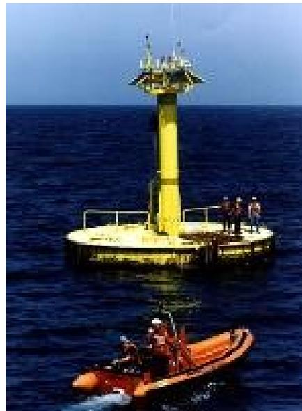
**Figure 2-3: 10-Meter Discus-Shaped Hull Buoy**
