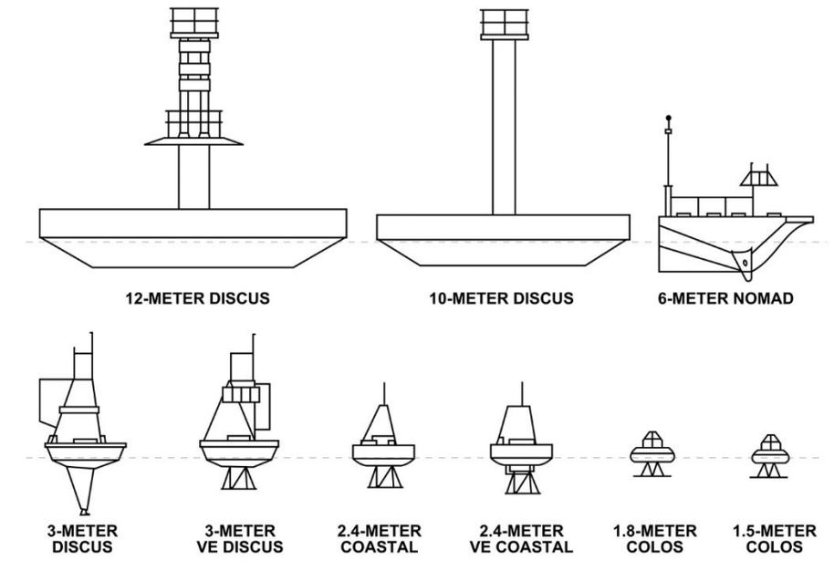
**Figure 2-2: Buoy Schematic**
