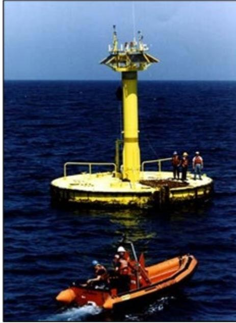
**Figure 2-3: 10-m Discus-Shaped Hull Buoy**
