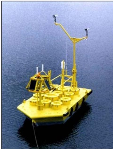
**Figure 2-4: 6-m Boat-Shaped Hull Buoy**
