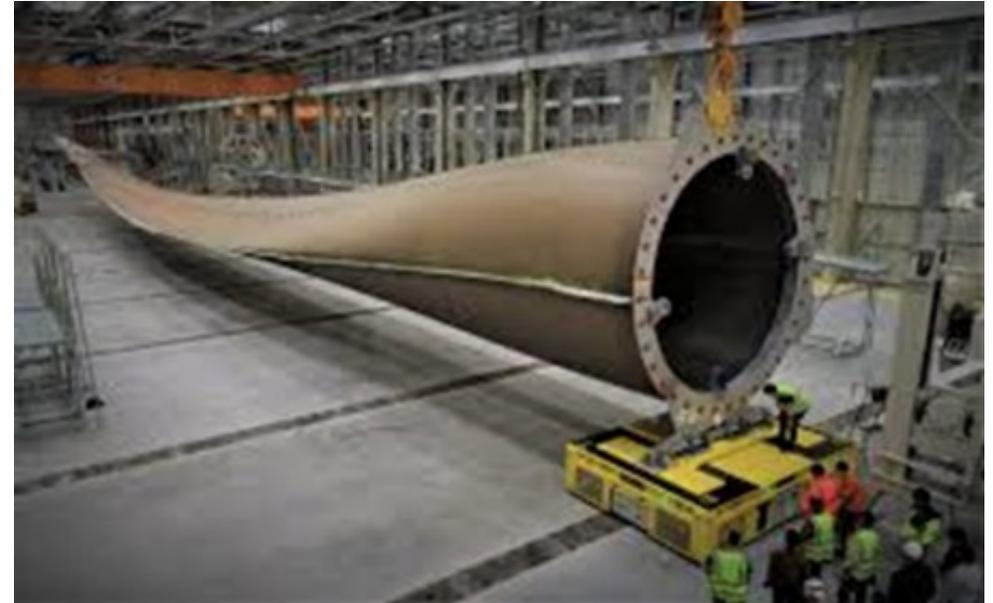
**107-meter Blade for GE 12-MW Wind Turbine**
