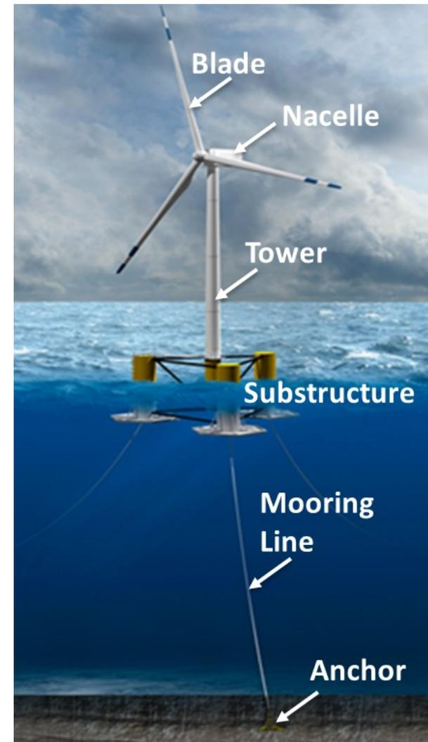
Parts of a Floating Offshore Wind Turbine NREL | 5
