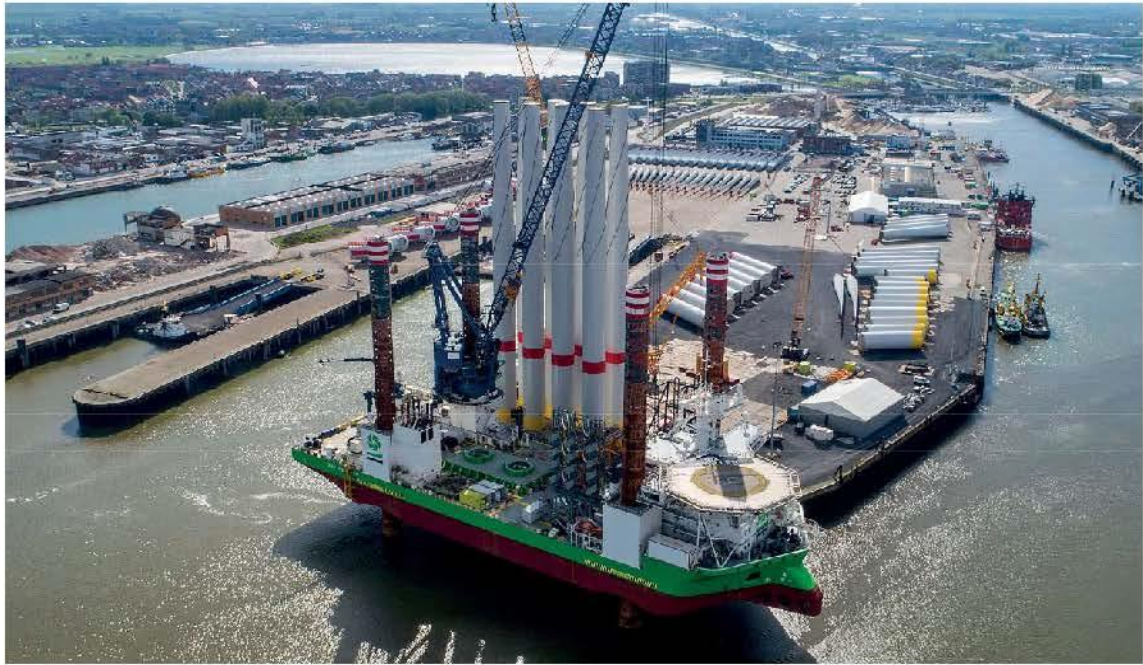
Transport of WTG Components via Jack-Up Vessel
