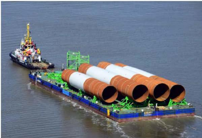
Monopile Transport via Tugboat and Barge
