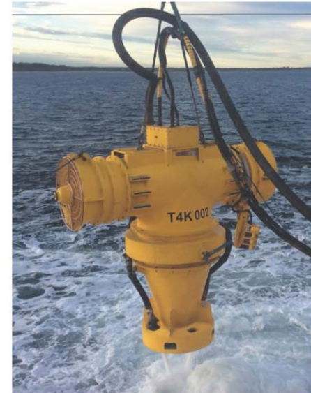
Controlled Flow Excavation
