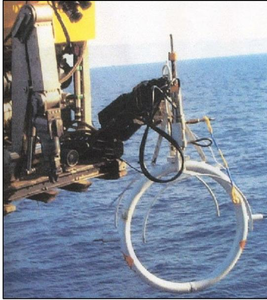
**FIGURE A-8 Externally deployed LSC mounted to ROV (JRC 2002)**
