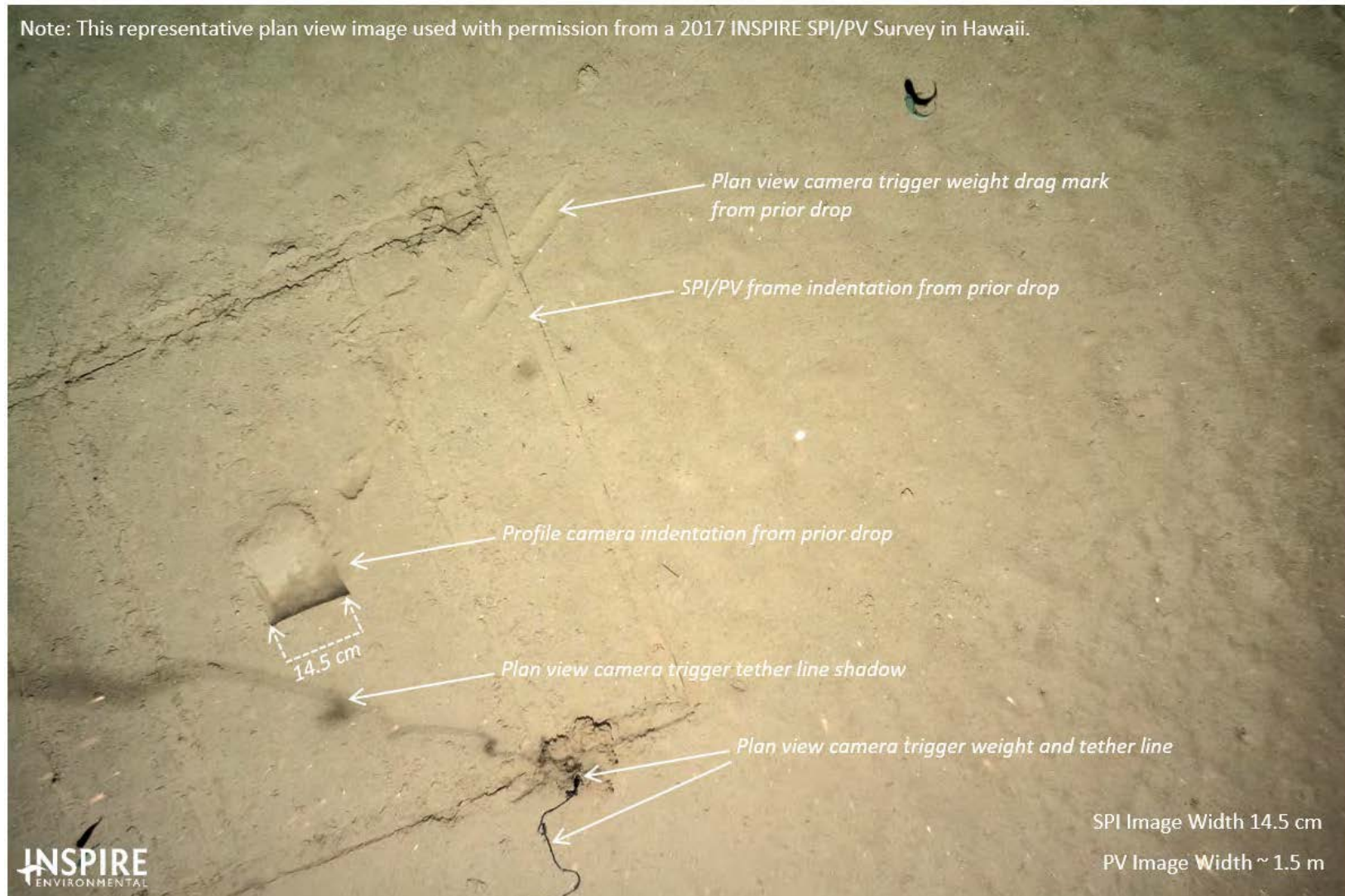
Figure 2-4. This representative plan view image shows the sampling relationship between plan view and sediment profile images. Note: plan view images differ between surveys and stations and the area covered by each plan view image may vary slightly between images and stations.
