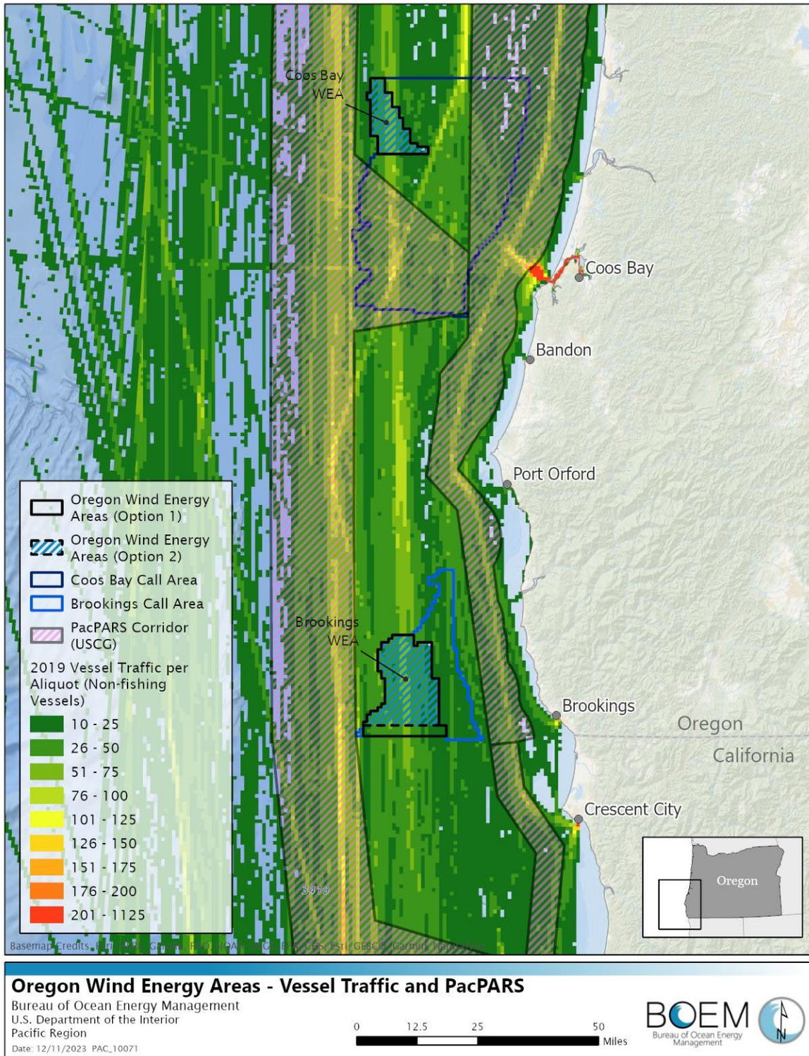
Figure 13: Map of Coos Bay and Brookings WEA Options overlaid with Automatic Identification System (AIS) data for all ship traffic traveling through an aliquot (1.2 x 1.2 kms) in 2019 and USCGRouting Map
